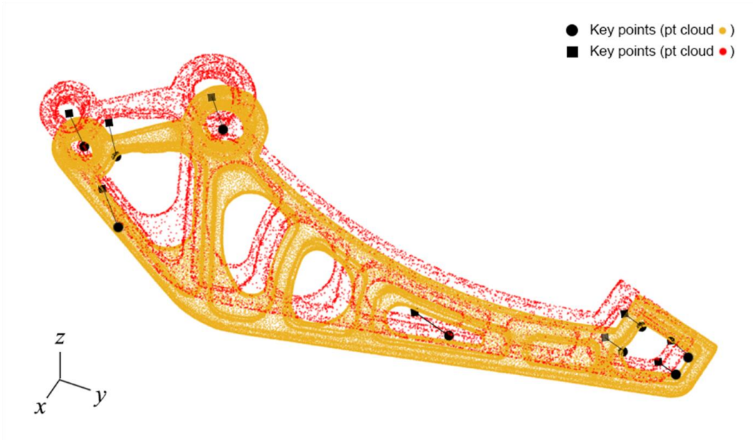
Figure 2.28 Paired of correspondences (squares and circles) identified in two point clouds (red and orange respectively) are matched via RANSAC alignment
