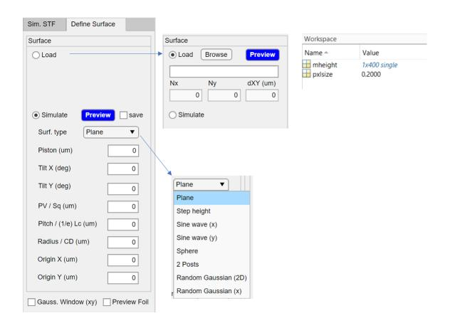
Choose an appropriate value for <No. point X>; click <Preview> to visualise the surface topography/profile. Tick <save> to save the visualised surface data. Tick <Preview Foil> to visualise the foil model of the surface and the corresponding spectrum. Tick <Gauss. Window (xy)> to add a lateral Gaussian window on the foil model to reduce its amplitude to nearly zero at the end of the FOV.
