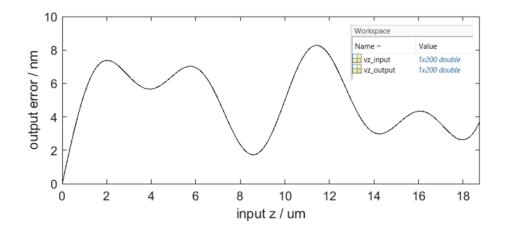
Click <Browse> to load the linearity data. Click <Preview> to visualise the linearity error. Switch on to enable the effect of linearity.
