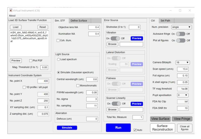
Go to <Define Surface> tab, choose Random Gaussian (2D) and set the Sq and Lc values, check <save> box, change <No. point X> to 1000, and click <Preview> to visualise and save the simulated surface data. Note that the 3D STF will be automatically resized to match the number of surface points.
