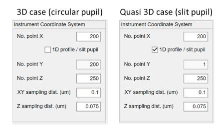
Once the 3D STF is generated and loaded (see section 0), the XY and Z sampling distances cannot be changed, but the number of points can be increased or decreased depending on the desired field of view (FOV) and scan length.
