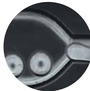
Particles being produced on the microfluidics T-junction chip.
