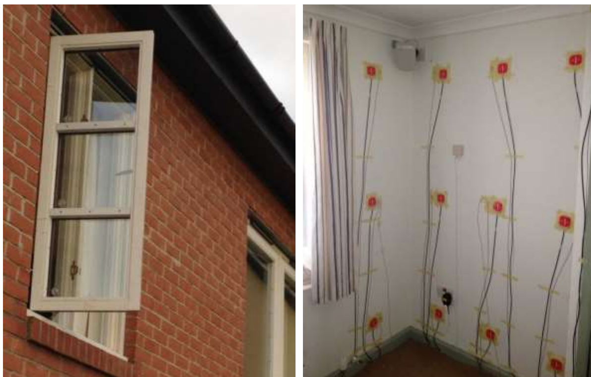
Figure 6: Vacuum glazing (left) and aerogel blanket internal wall insulation solution (right) tests at the E.ON retrofit research house
