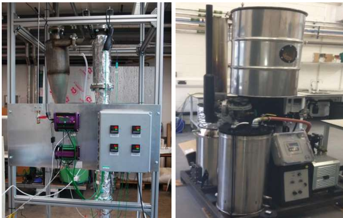
Figure 5: Fluidized bed reactor for carbon capture with solid sorbents(left) and 10kW biomass-gasification based power generator (right)
