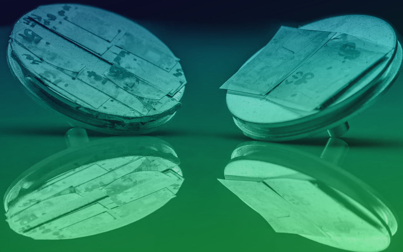
Image: Interface patterns between water-soluble and structured inks were designed and inkjet printed before applying FIB-SEM and OrbiSIMS analyses.
