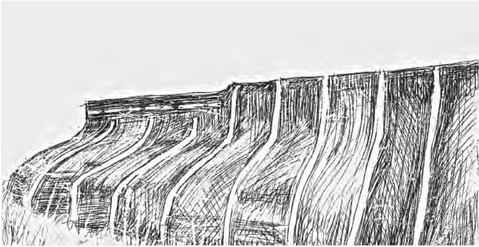
Fig. 15. Artist's sketch of an overturned coble, showing the Norse-style shallow bottom. Illustration by Jo Shortt Butler.
