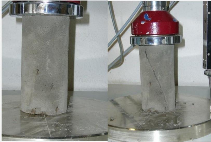
Figure. 2. An example of a solidification sample of fluidised bed combustion ash—the sample showed a semi-rock character during the compressive strength test (50kN).
