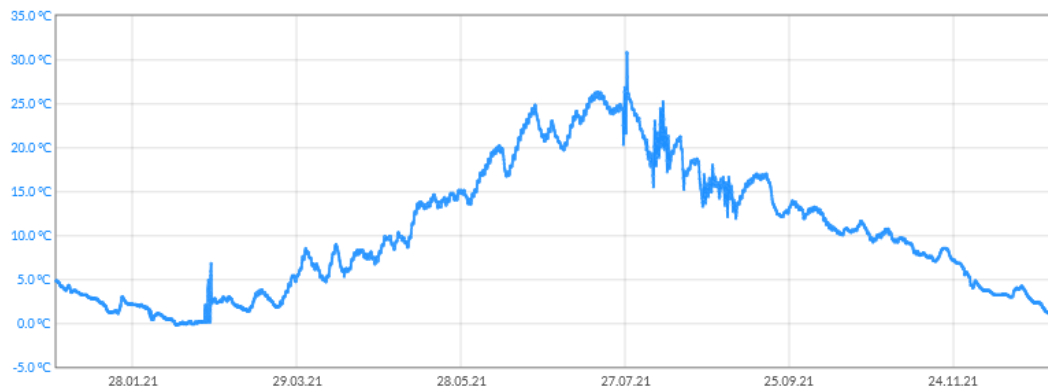
Figure 6.11. Ground temperature plot (-50cm) recorded in 2021 at the heap of LW Bogdanka mine, E Poland
