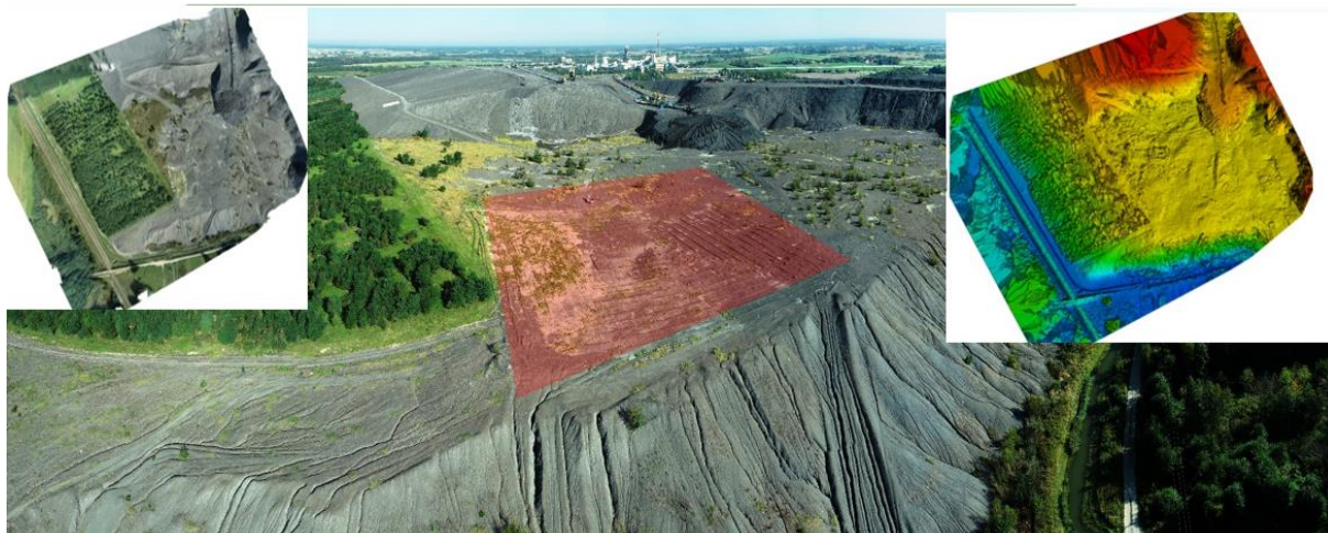
Figure 6.12. View of the scanned area of the LW Bogdanka mine, E Poland - a fragment of the dump was inventoried in 3D using laser scanning and low-level photogrammetry, carried out with the use of drones.
