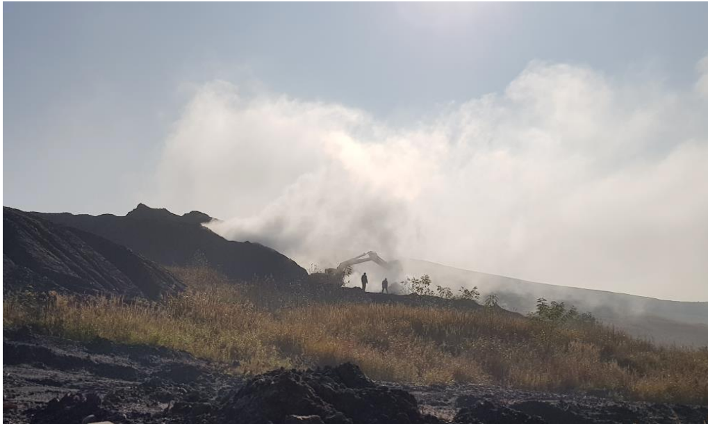
Figure 3.6. Endogenous fire of the spoil in Libiąż town, S Poland (Image courtesy of GIG).
