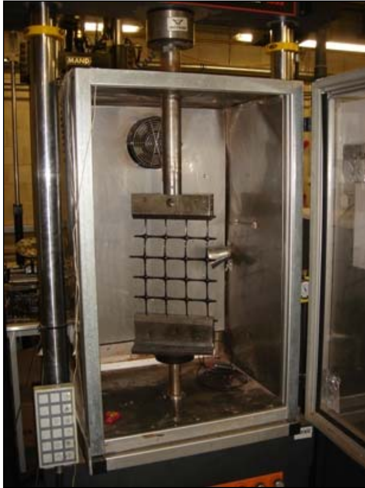
Figure 3.18 Geogrid stiffness test arrangements in Instron
