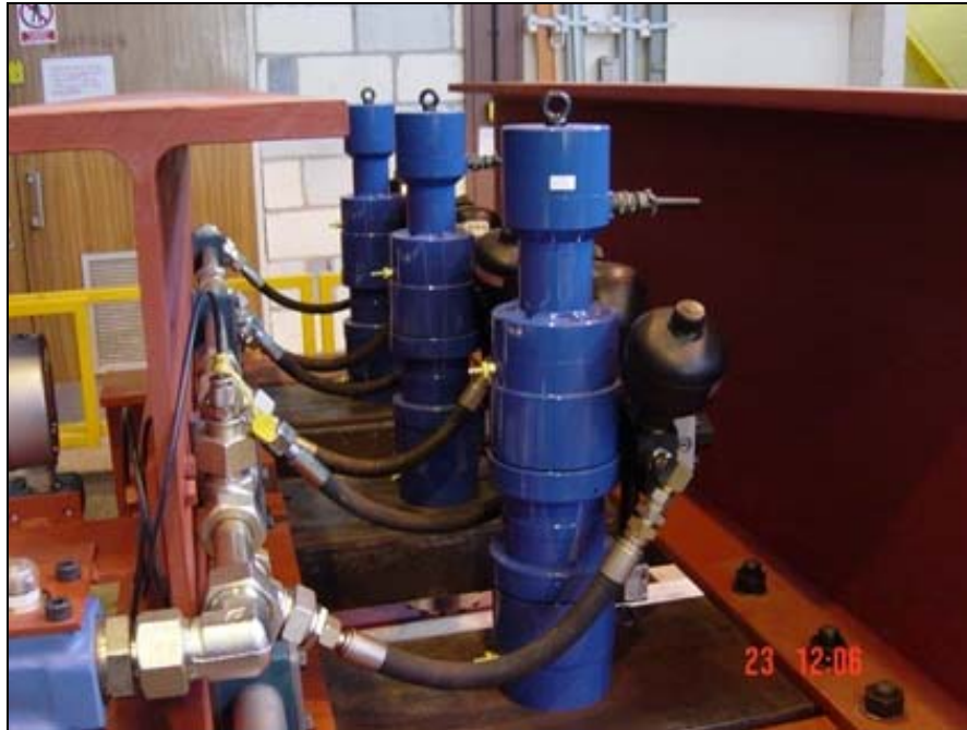
Figure 5.10 Servo controlled hydraulic actuators
