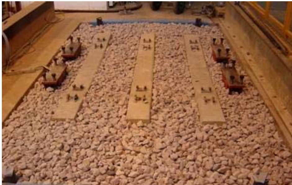
Figure 5.7 Sleepers level with the top of ballast
