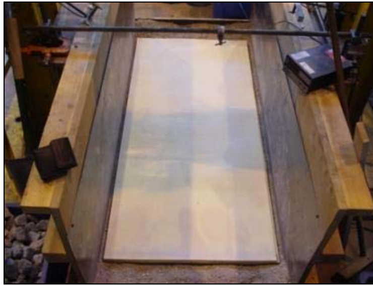
Figure 4.4 Rubber subgrade in CET
