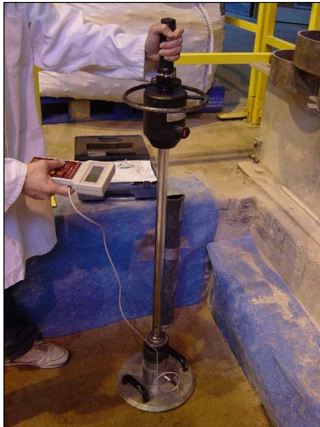
Figure 5.6 German Dynamic Plate measuring subgrade stiffness
