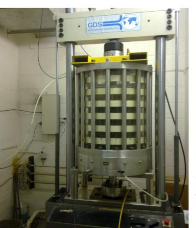
Large scale triaxial test to measure the effect of stress levels on the performance of clean ballast
