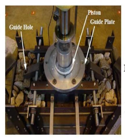
Box tests to consider the effect of maintenance on the performance of dirty ballast
