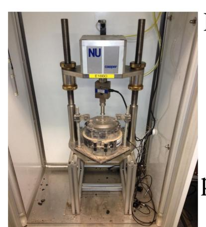
PUMA tests to measure the effect of fouling and water on the performance of dirty ballast
