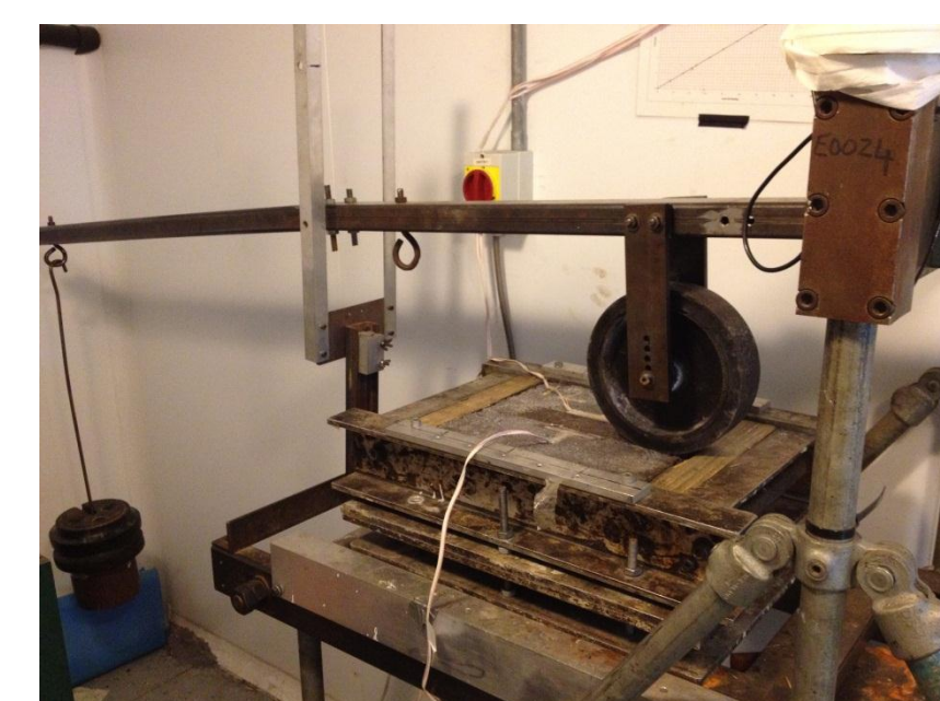
Figure 2: Wheel Tracking Device and finally Sample Surface
