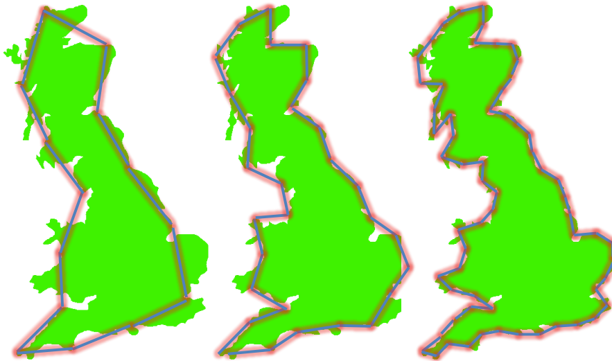
Figure 2.18 Coastline of Great Britain measured using successively smaller units
