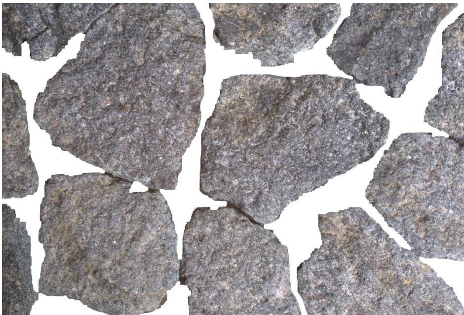
Figure 4.10 Dolerite aggregate photograph masked to segregate aggregate from sand-filled gaps
