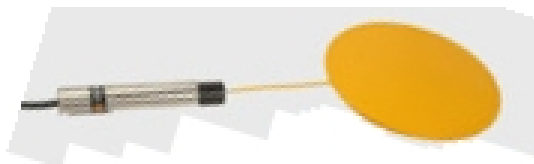
Figure 5.9. Vibrating Wire Pressure Cells.
