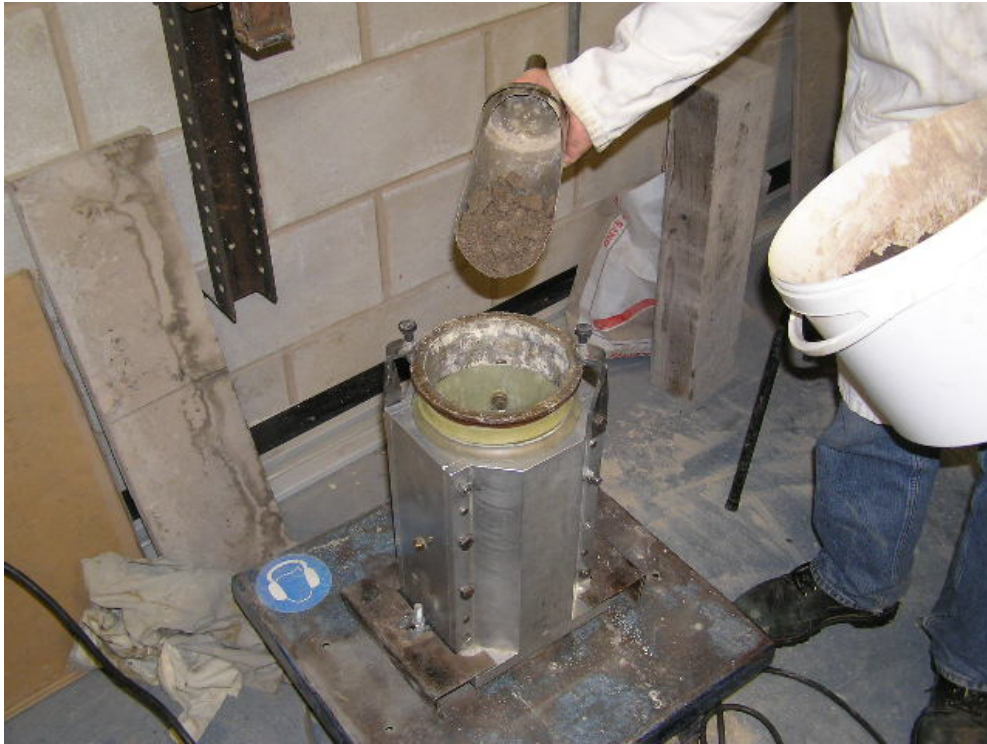
Figure 3.7. Adding material to compaction mould for RLT sample preparation.
