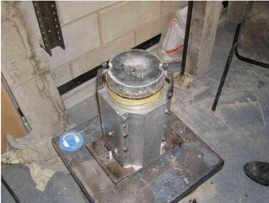
Figure 3.9. The use of the end platen to ensure the correct finished height for the final layer.
