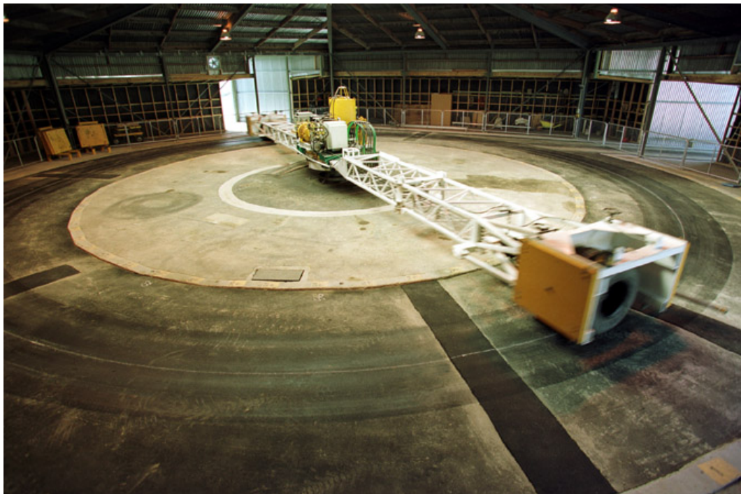
Figure 4.1. Transit New Zealand's pavement testing facility CAPTIF.
