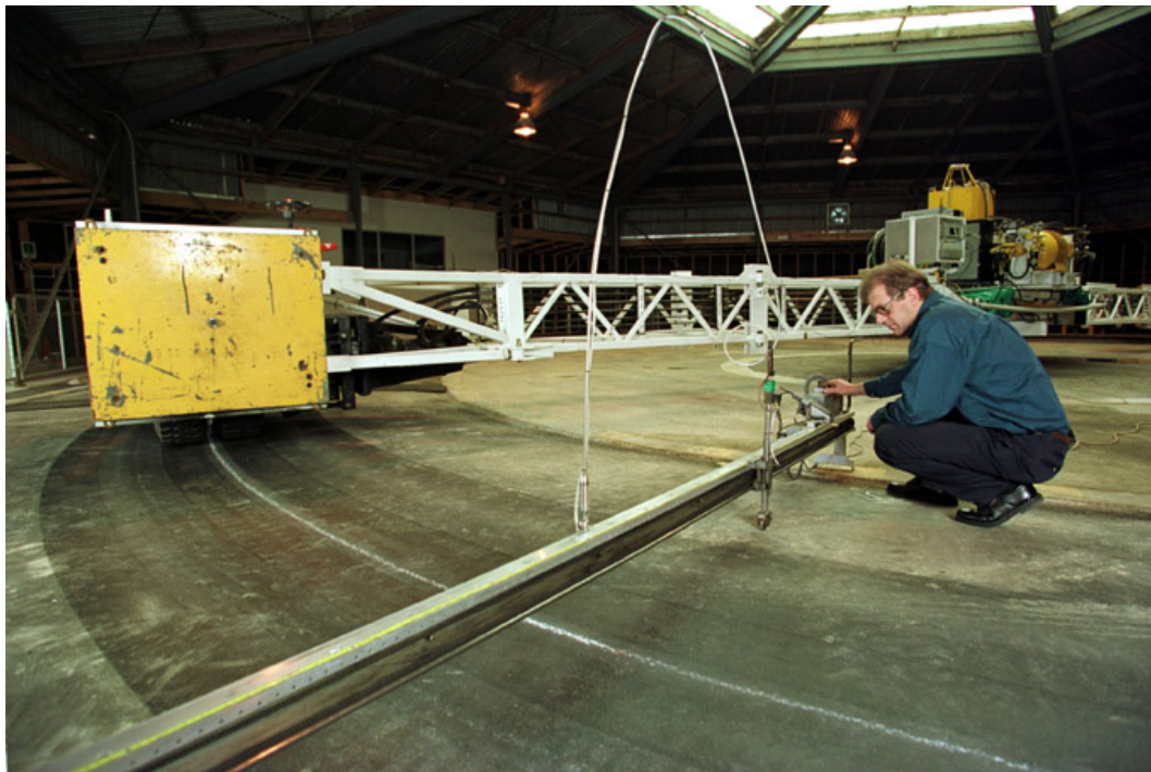
Figure 4.9. Transverse profile measured using the CAPTIF profilometer.
