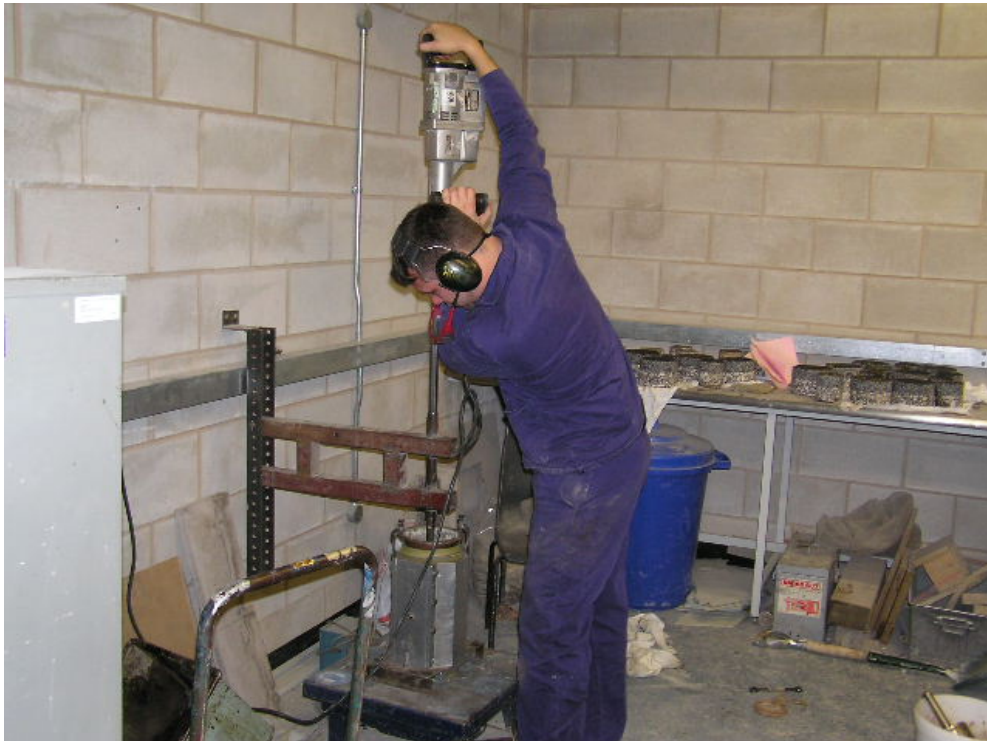
Figure 3.8. Compacting material layers for RLT sample preparation.
