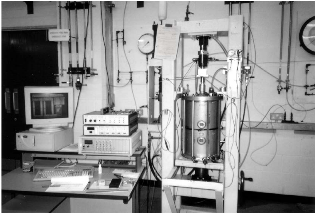
Figure 3.1. University of Nottingham Repeated Load Triaxial (RLT) apparatus.
