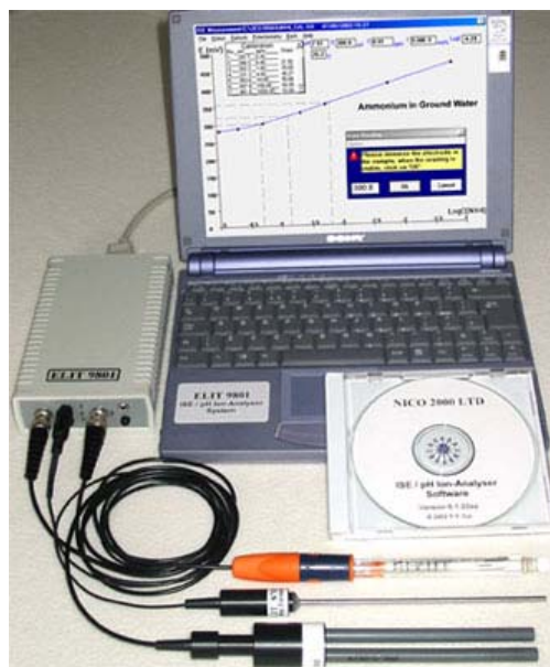
Figure 3.4, Equipment used for ion selective electrode analysis. Taken from www.nico2000.net .
