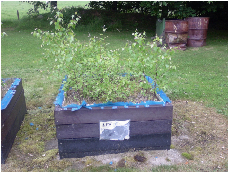
Figure 3.1, Photo showing plant growth in the lysimeter containing municipal solid waste incinerator ash.
