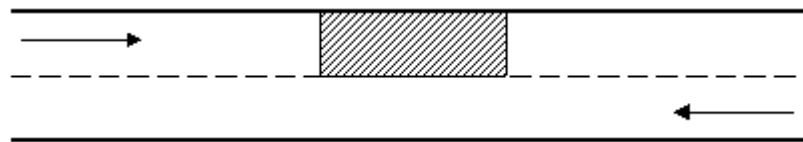
Figure 3-10: Single carriageway road with shuttle working
