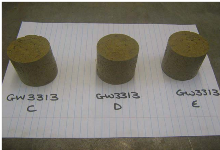
Figure 10. L-TPS-10B material with 1.5% lime, European accelerated swelling test specimens, 0% volume change:
