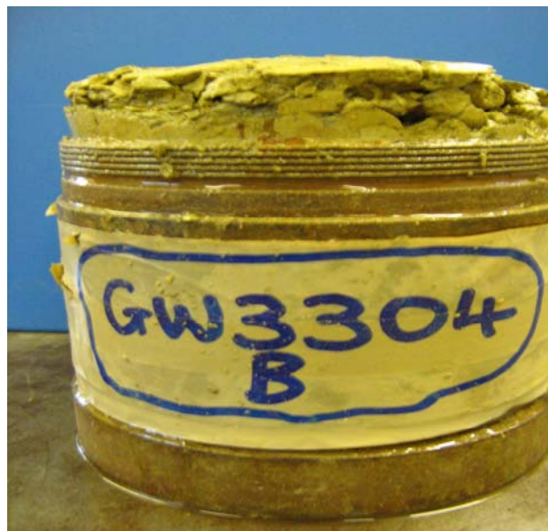
Figure 8a: 7 day CBR specimen, mix H-TPS-7A
