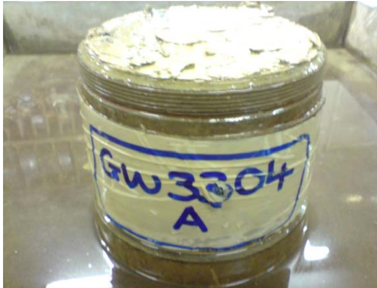
Figure 8a: 7 day CBR specimen, mix H-TPS-7A
