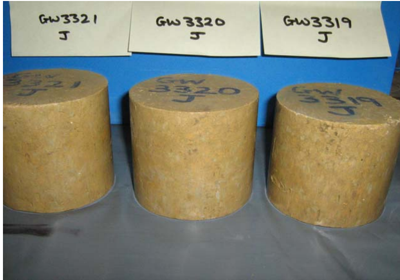
Figure 9. L-TPS-12B material with 1.5% lime and 3% (14 days air curing and 14 days soaking), MCV specimens, loss of strength = 32%, 0% volume change:
