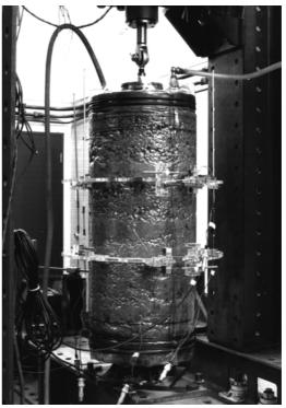
Constant Confining Pressure Apparatus (200 mm x 100 Ømm) for Testing of Subgrade Soils
