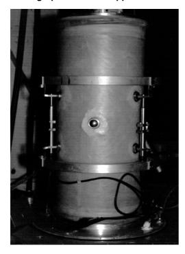
Variable Confining Pressure Apparatus (320 mm x 160 Ømm) for Testing Unbound Granular Materials
