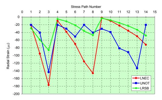
Figure 7-6 Comparative Strain Reading Normalised with Deviator Stress Paths for a Specimen of Hard Limestone
