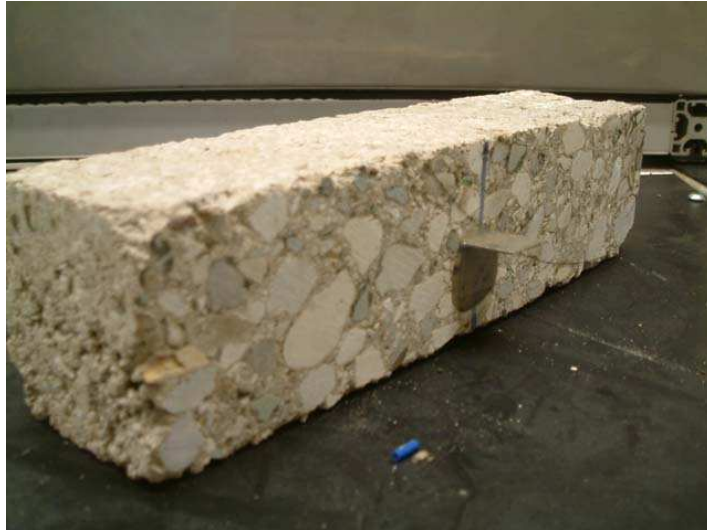
Figure 5.8 Beam specimen for four-point bending test
