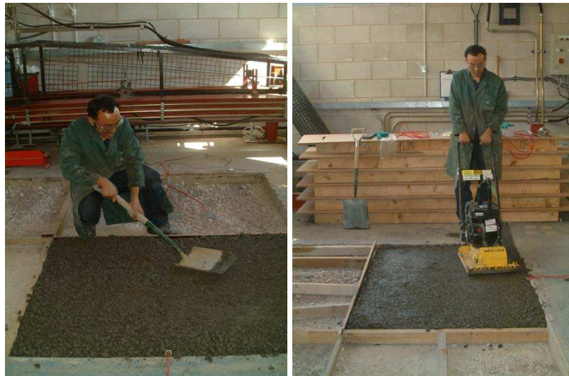
Figure 6.13 Spreading and compacting the material in PTF pit
