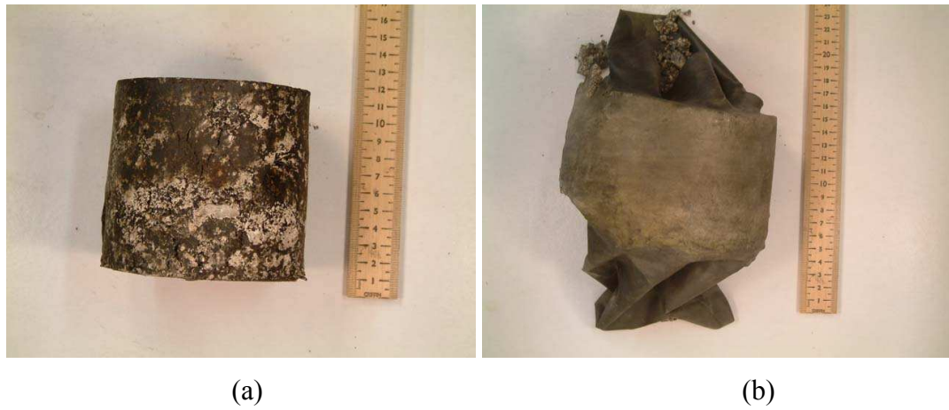
Figure 4.7 Specimen failure (a) at cyclic stress = 400 kPa (b) at cyclic stress = 800 kPa
