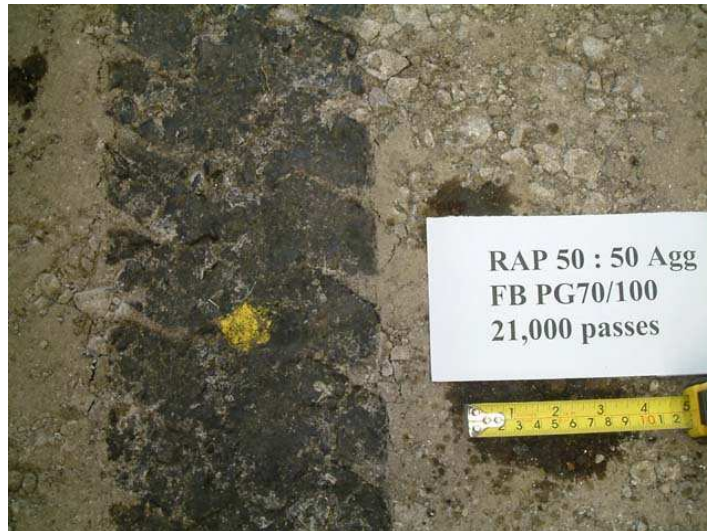
Figure 6.16 Observed longitudinal cracks at both sides of the wheel path on the foamed bitumen stabilised pavement
