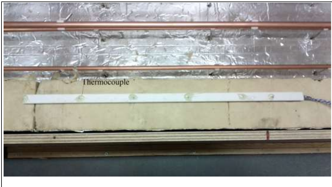
Figure 5-8 Thermocouples were fastened on a conduit
