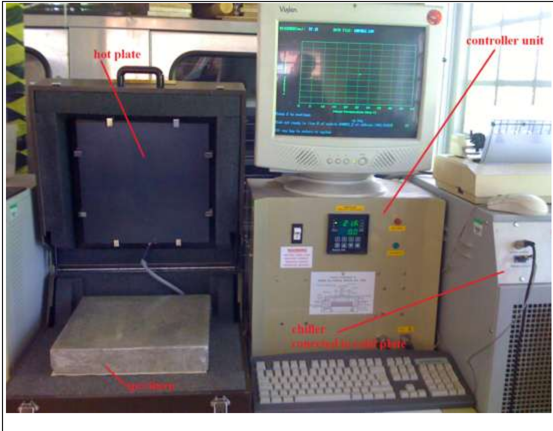
Figure 3-2 Heat flowmeter apparatus for thermal conductivity measurement
