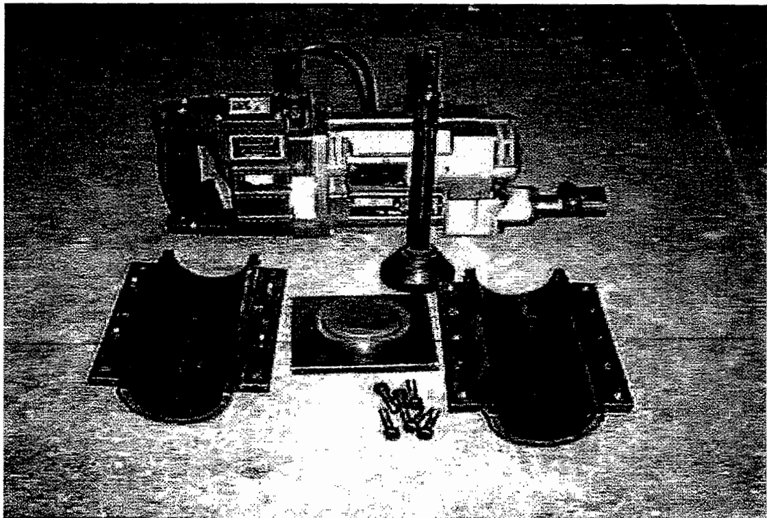
Figure 4.2 Photograph showing split mould and Kango compactor.
