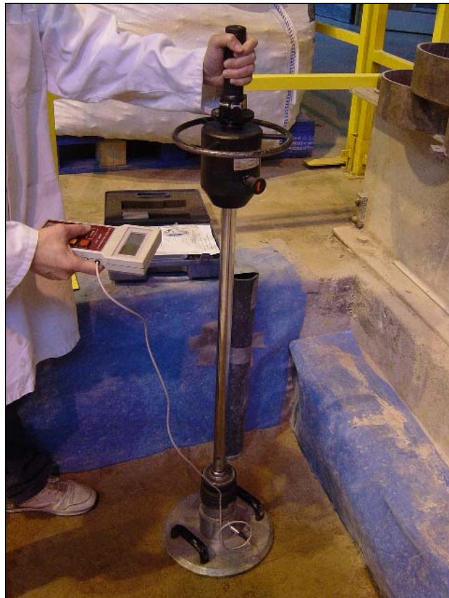
Figure 5.6 German Dynamic Plate measuring subgrade stiffness
