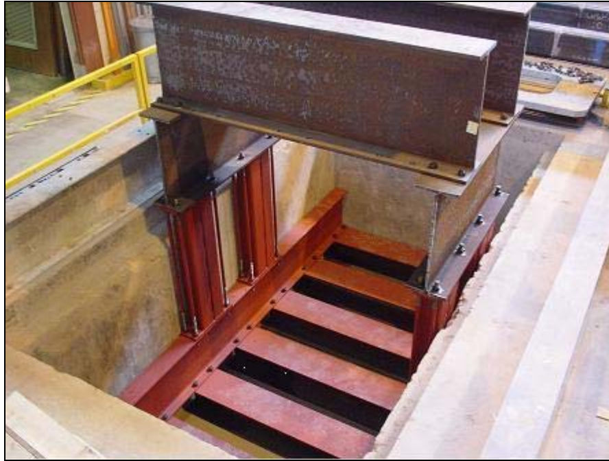
Figure 5.2 Steel frame in concrete lined pit for RTF
