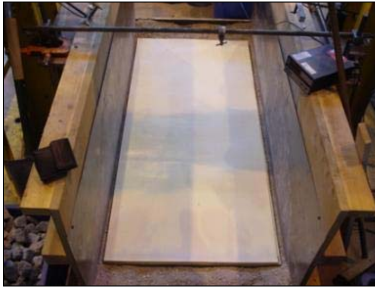
Figure 4.4 Rubber subgrade in CET
