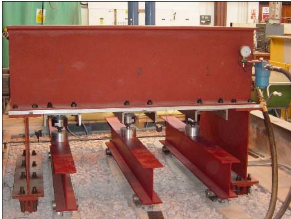
Figure 5.9 RTF loading arrangement
