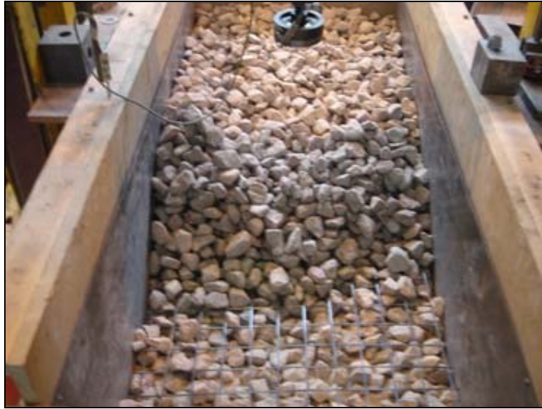
Figure 4.6 Grid sitting on a single layer of ballast (CET)
