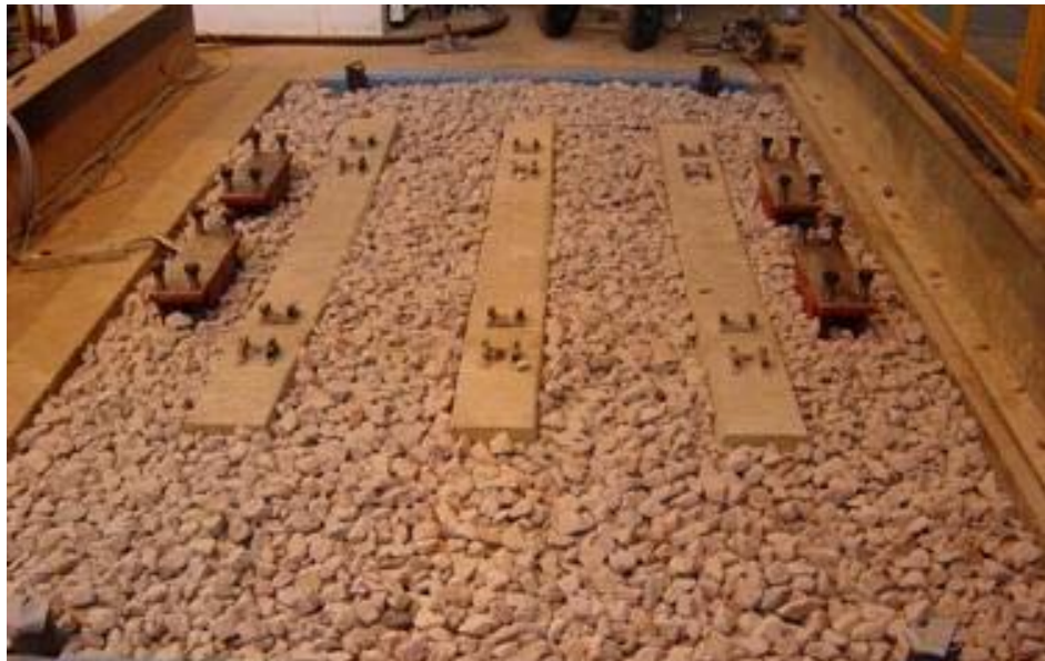
Figure 5.7 Sleepers level with the top of ballast
