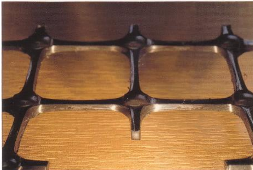
Figure 2.26 Physical attributes of a Tensar biaxial grid (Tensar International, 2001)
