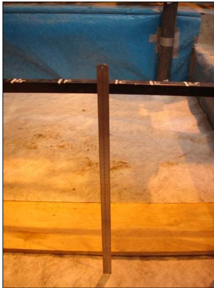
Figure 5.15 Measurement of subgrade settlement
