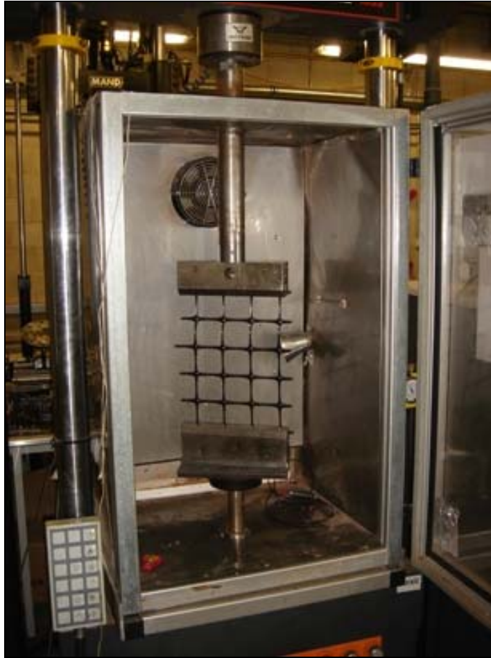
Figure 3.18 Geogrid stiffness test arrangements in Instron
