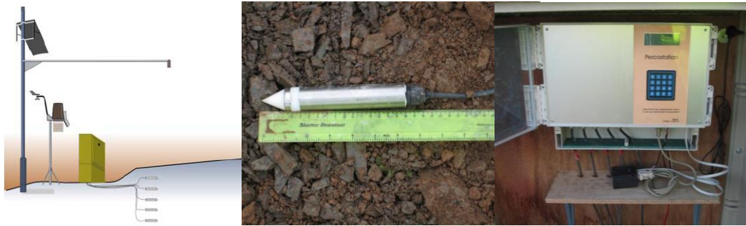
Figure 3.7 – (a) Schematic diagram of a Percostation Installation [Saarenketo & Aho 2005] (b) Percostation's Probe (c) Percostation System
