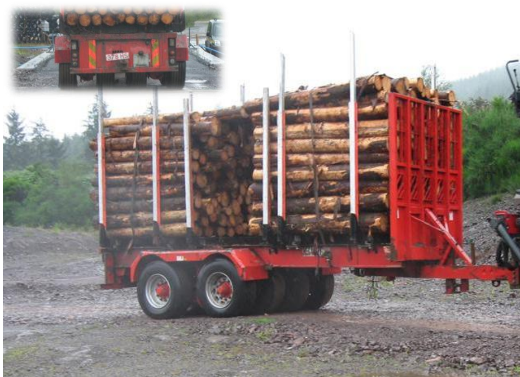
Figure 4.24 – “Low ground pressure” vehicle trailer with tyres equally spaced across pavement on stub-axes
