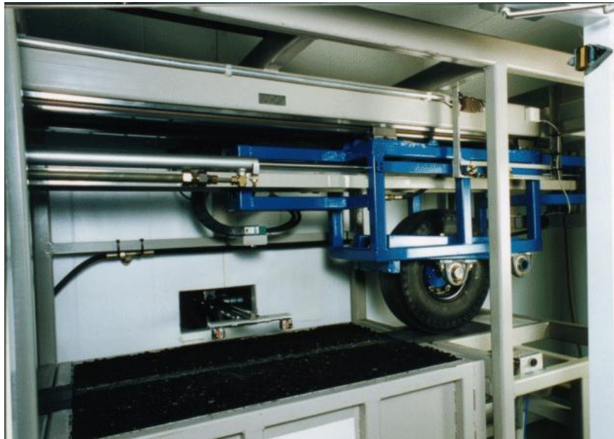
Figure 2.18 – Wheel tracking test equipment at the University of Oulu – Finland
