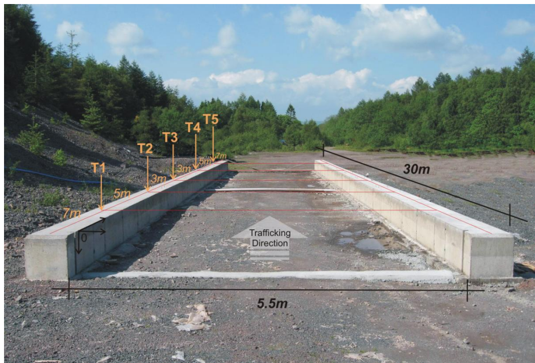
Figure 4.13 – Ringour Testing Facility before construction of the test section with major dimensions indicated and sections chainage
