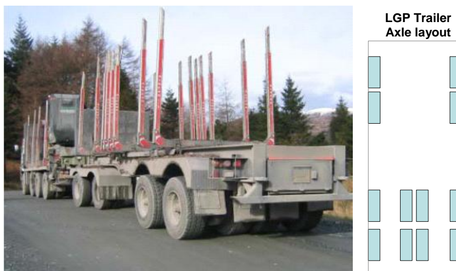
Figure 3.4 – Low ground pressure vehicle and its axle configuration
