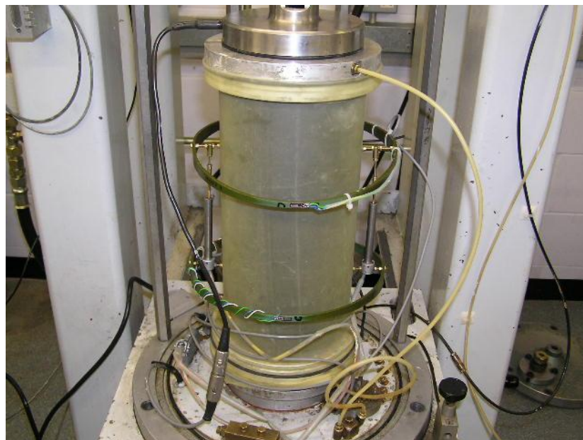
Figure 2.17 – Repeated load triaxial test equipment at the University of Nottingham
