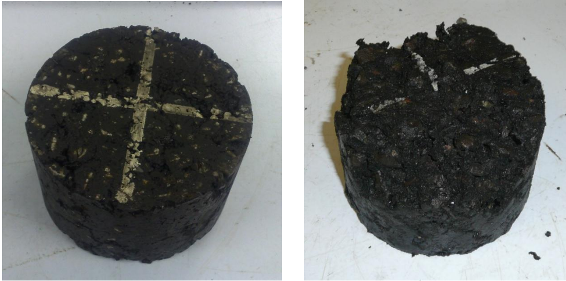
Figure 6.24 - Control specimen (left) and a 3 % addition of sodium silicate (right) showing the difference in edge deformation after 3 BBA HAPAS cycles.
