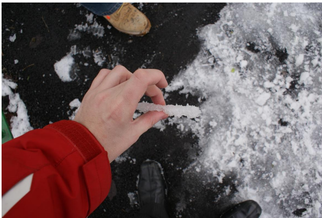
Figure 7.20 – Plate of ice that was easily removed from the anti-icing surface.
