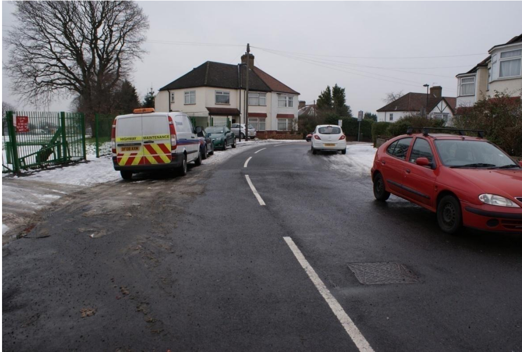
Figure 7.19 – Photograph showing less ice formation on anti-icing surface (front) and control surface (back) on the 12 th January 2010.
