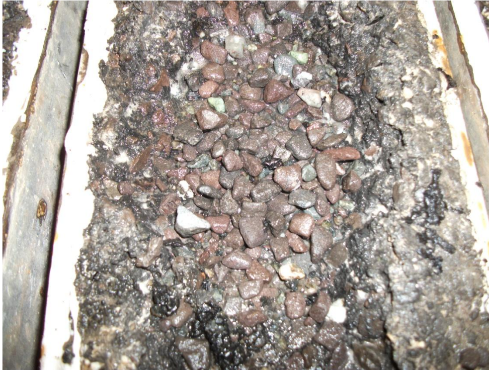
Figure 6.29 – Photograph demonstrating the stripping of surface aggregate on the 100% sodium silicate sample after 12 hours of wheeltracking
