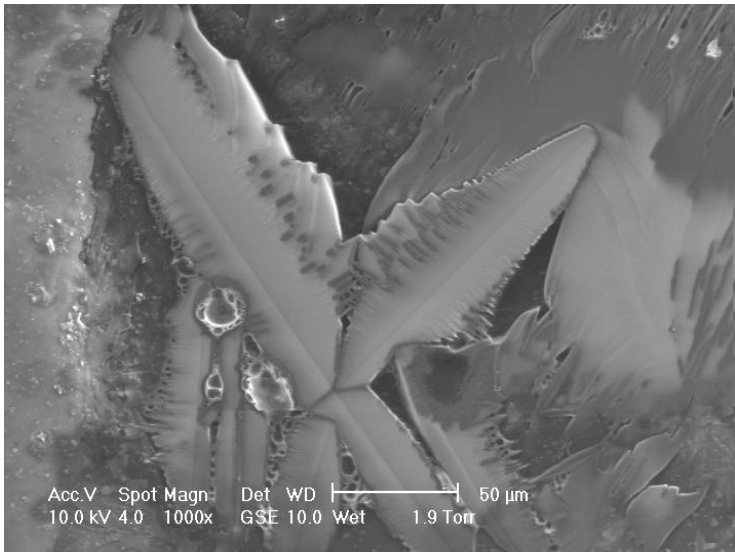
Figure 6.48 - Example of angular crystalline formation of deposited sodium formate
