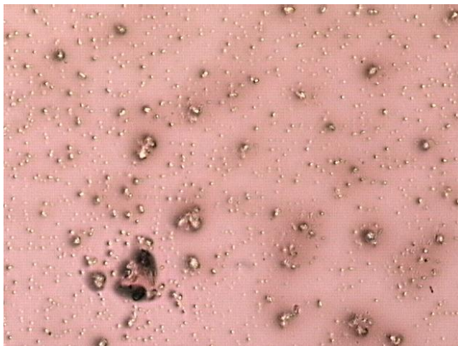
Figure 6.5 – Chemical formulation of 30% Sodium Formate 70% Sodium Silicate at a magnification of 10x.
