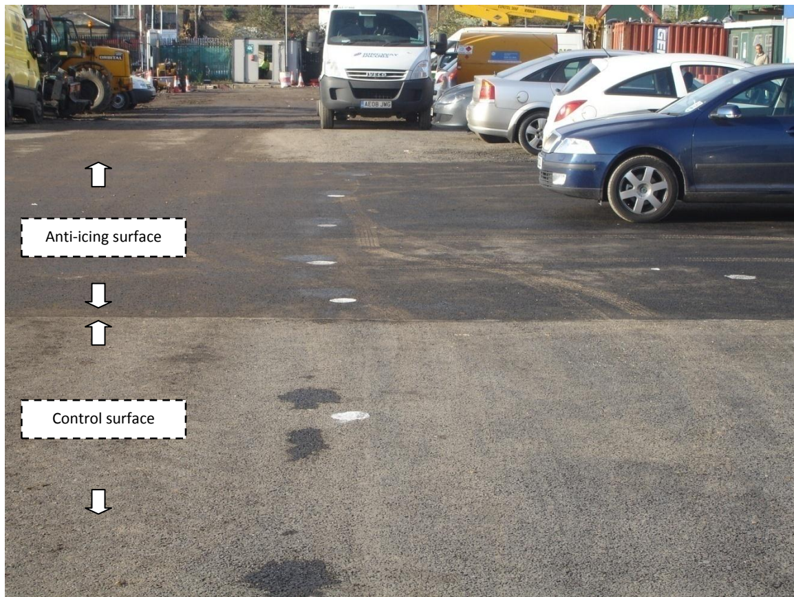
Figure 7.6 - Visual difference between surface courses due to moisture attraction damp anti-icing surface course (top) and dry control surface (bottom)
