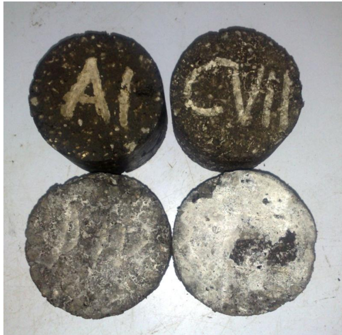
Figure 6.65 – Specimens after drying showing the control (top left), 100% sodium formate (top right), 50% sodium formate and 50% sodium silicate (bottom left) and 100% sodium silicate (bottom right)
