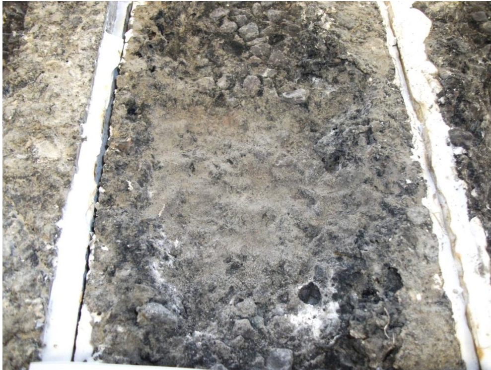
Figure 6.31 – Photograph demonstrating the disintegration and breakdown of aggregate structure of the 100% sodium silicate sample shown in Figure 6.29 after drying and the removal of loose aggregate
