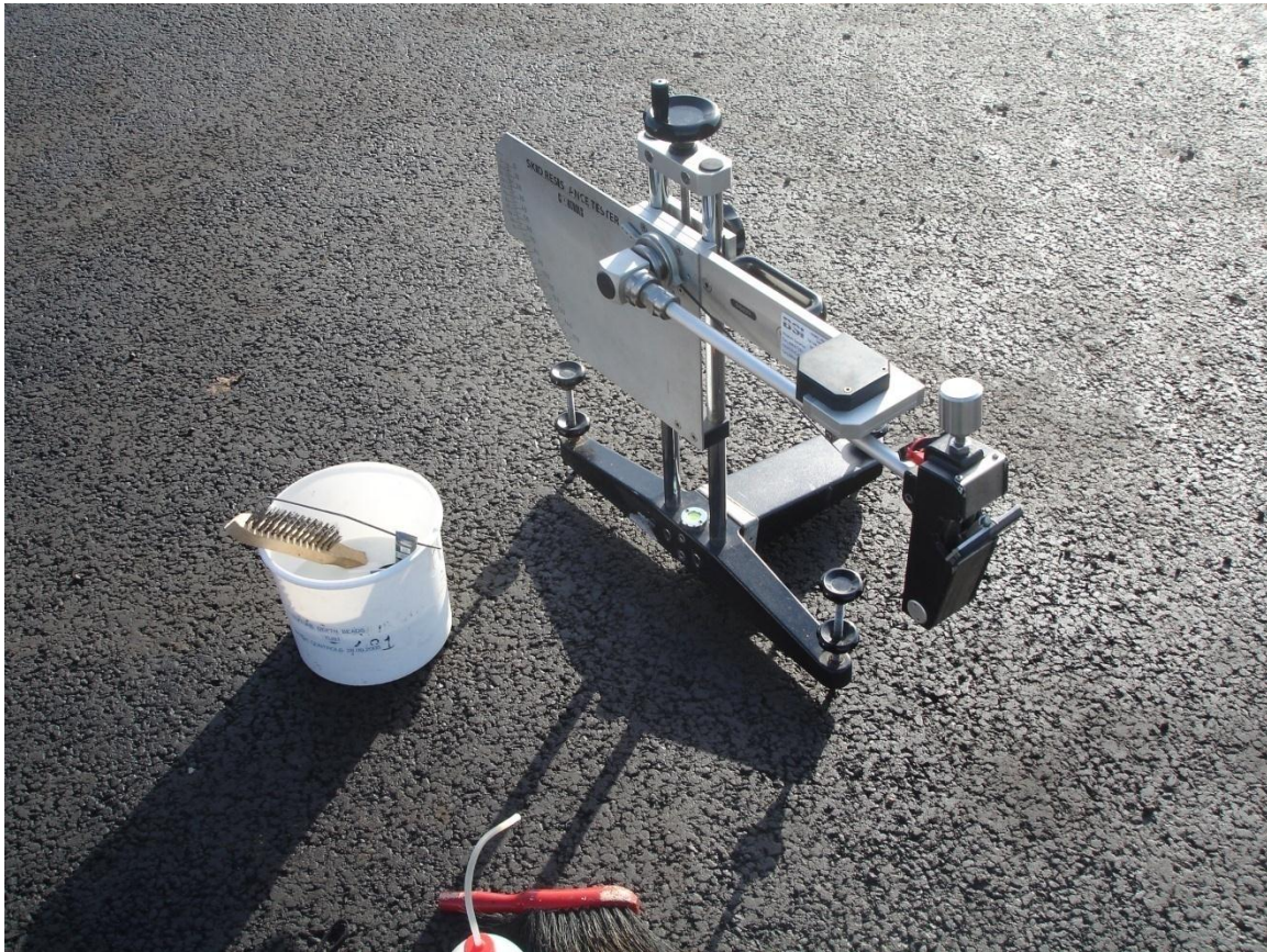
Figure 7.5 - Pendulum skid tester and volume patch equipment
