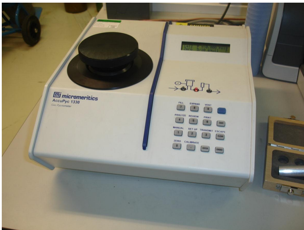
Figure 5.5 – Photographs of gas displacement pycnometer
