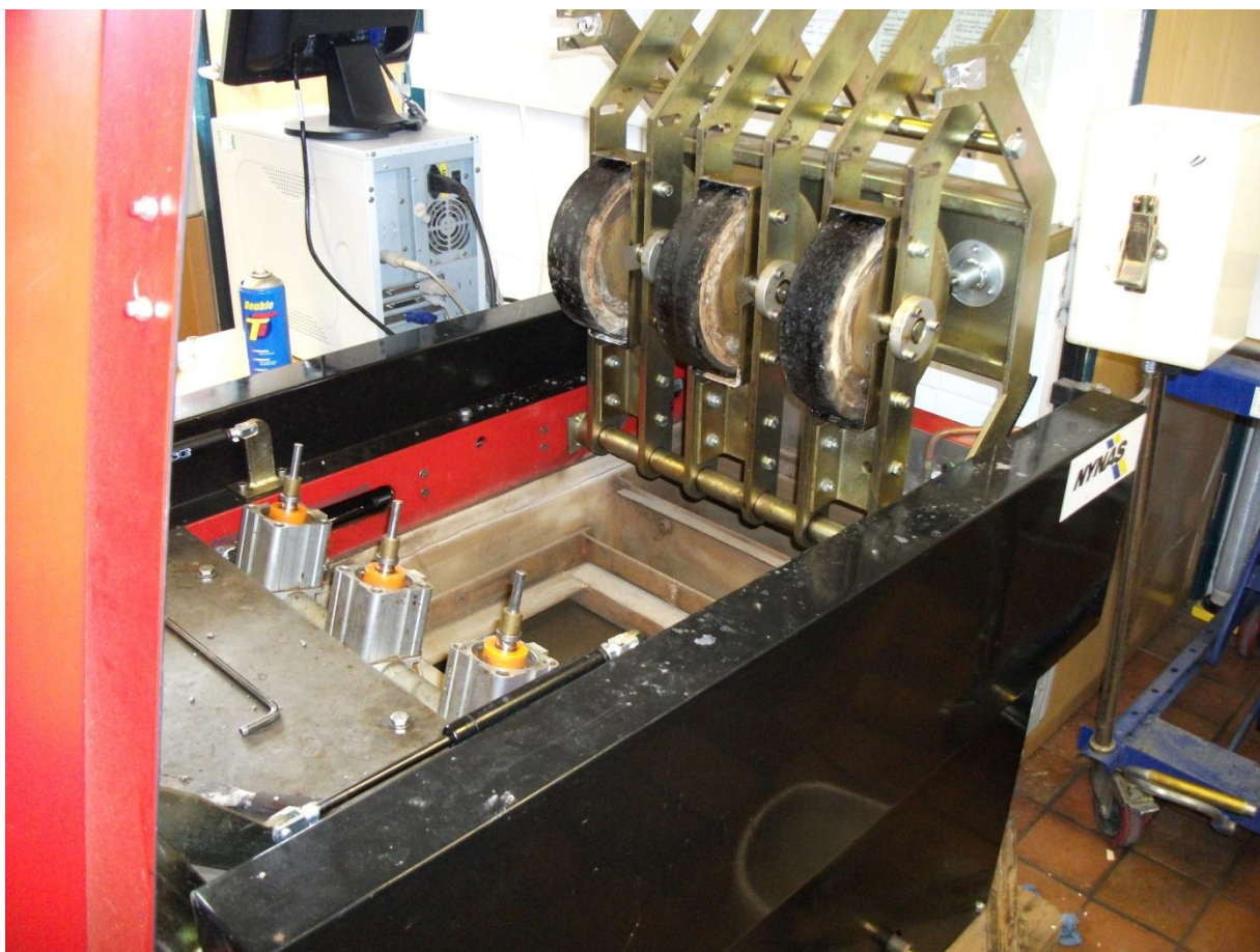
Figure 6.27 - Submerged wheeltracker equipment used for testing
