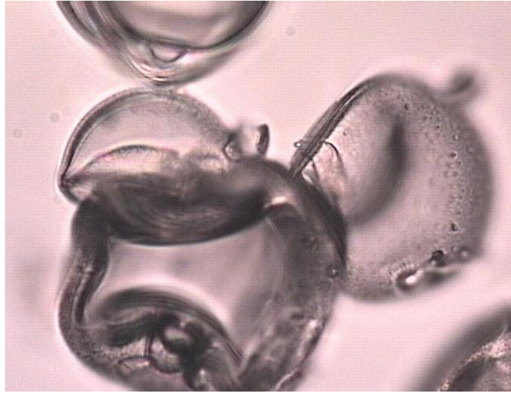
Figure 5.9 - Sodium Silicate at x20 magnification
