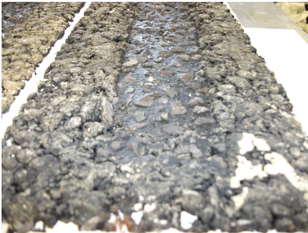
Figure 6.30 – Photograph of control sample surface after 12 hours of wheeltracking
