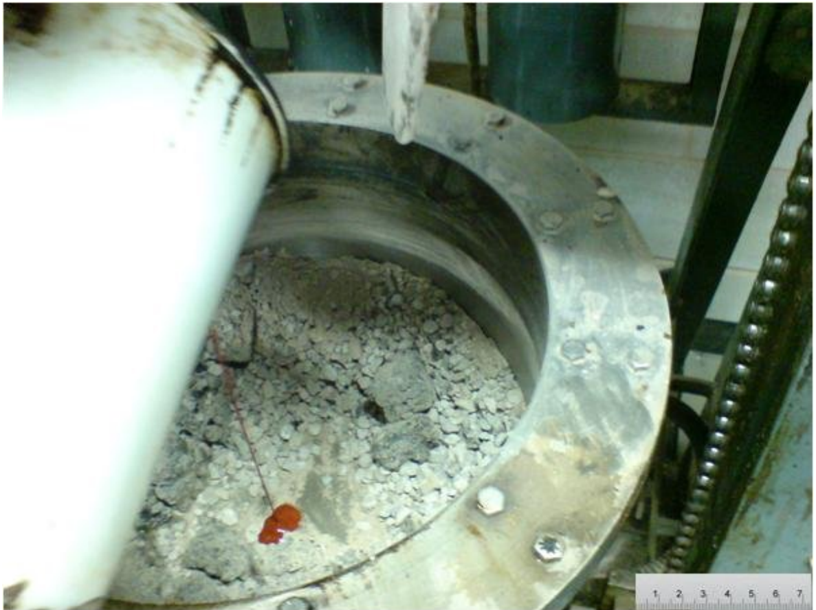
Figure 43: RAP size after 2 minutes RAP/superheated virgin aggregate mixing time
