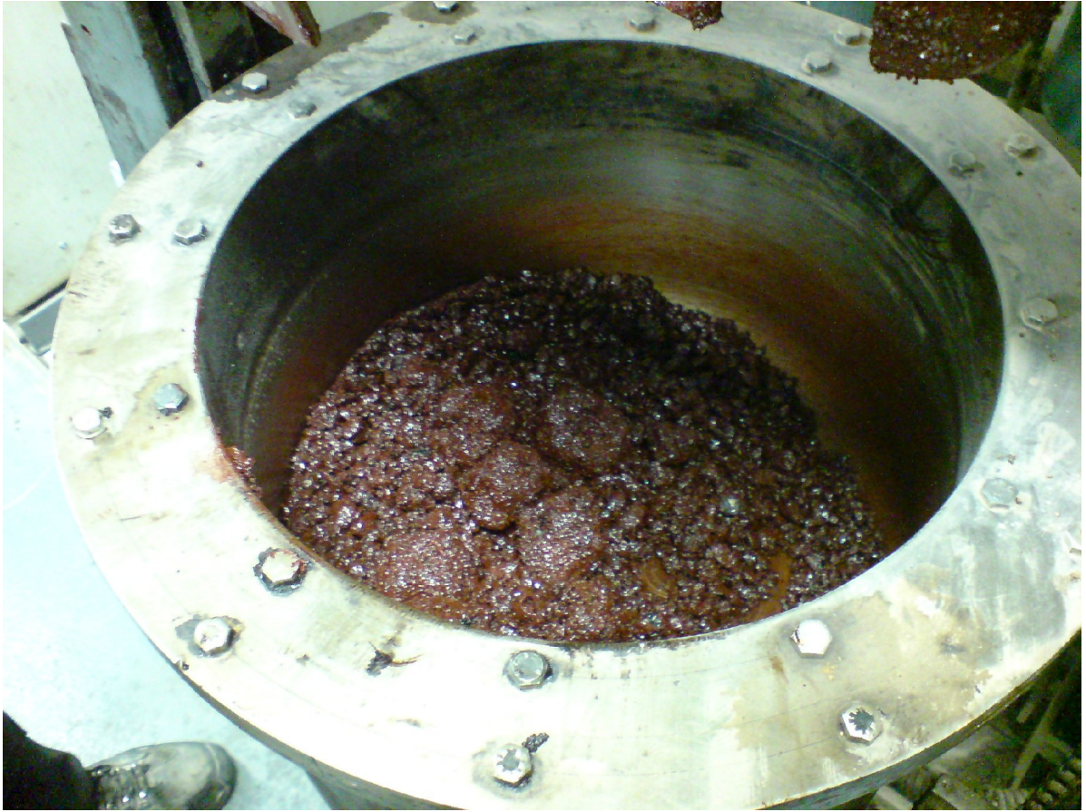
Figure 59: Small particles tend to move downward to the bottom during mixing process
