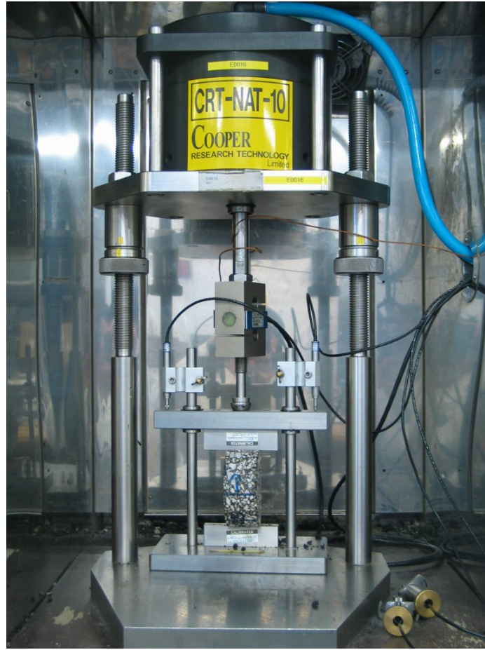
Figure 89: Schematic of ITFT test
