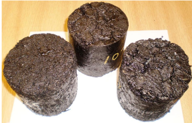
Figure 5.16 Specimen ready for compression testing
