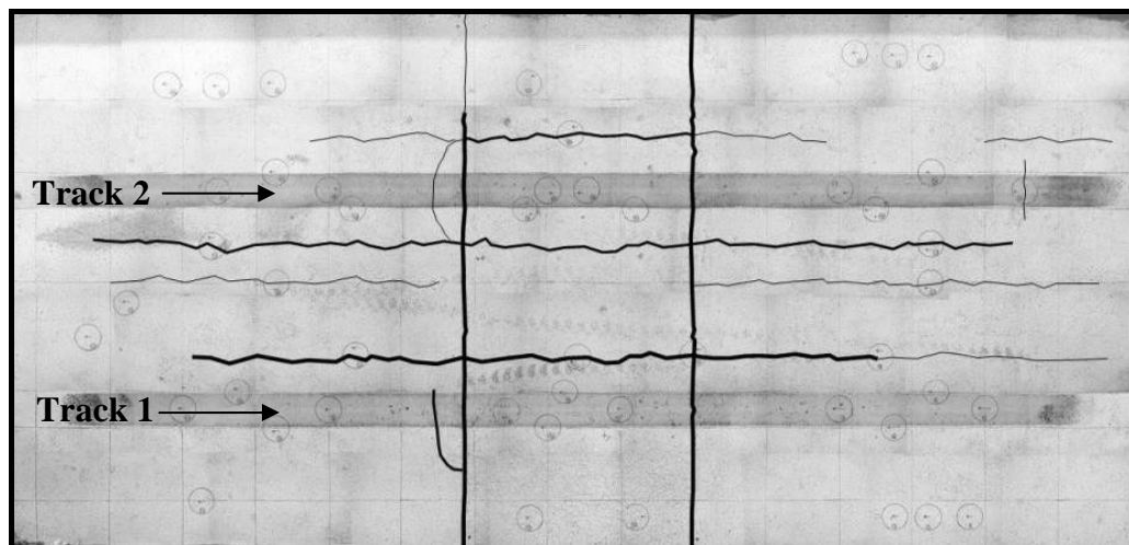
Figure 7.23 – Main cracks observed at the pavement surface at the end of the test
