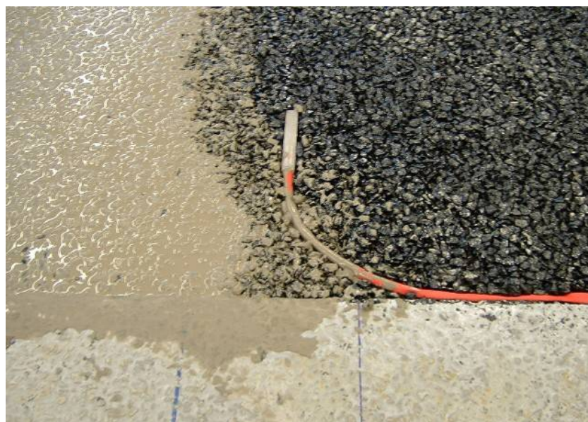
Figure 7.17 – Strain gauge located in the wheel path at the surface of the pavement
