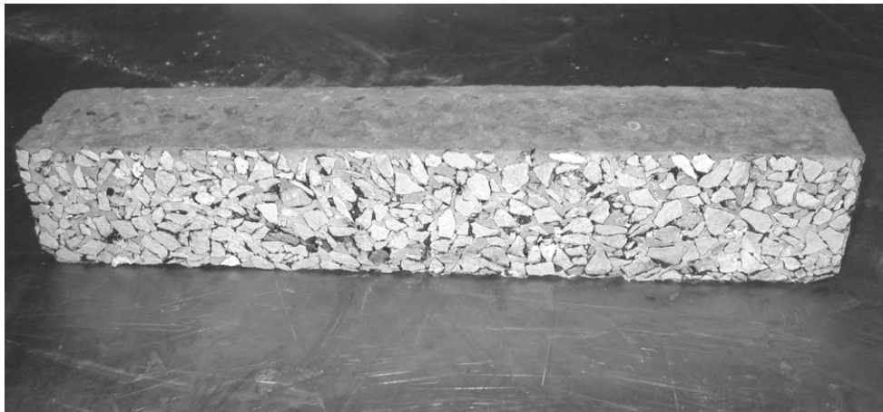
Figure 4.2 – Grouted macadam specimen to be used in the four-point bending test
