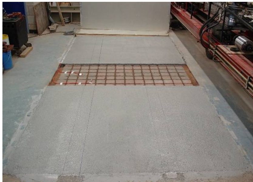
Figure 7.16 – Pavement construction prior to the application of the porous asphalt in the last section
