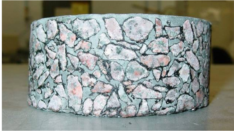
Figure 5.3 – Ø100 mm specimen obtained with full penetration of grout
