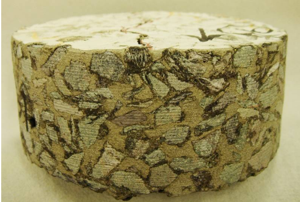
Figure 7.29 – Core extracted from PTF middle section
