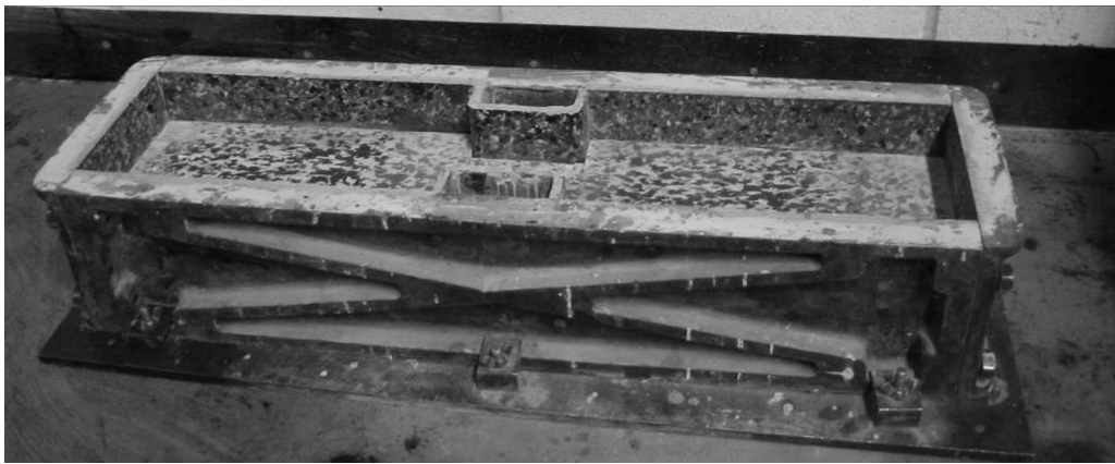
Figure 6.25 – Mould used to manufacture thermal cracking specimens
