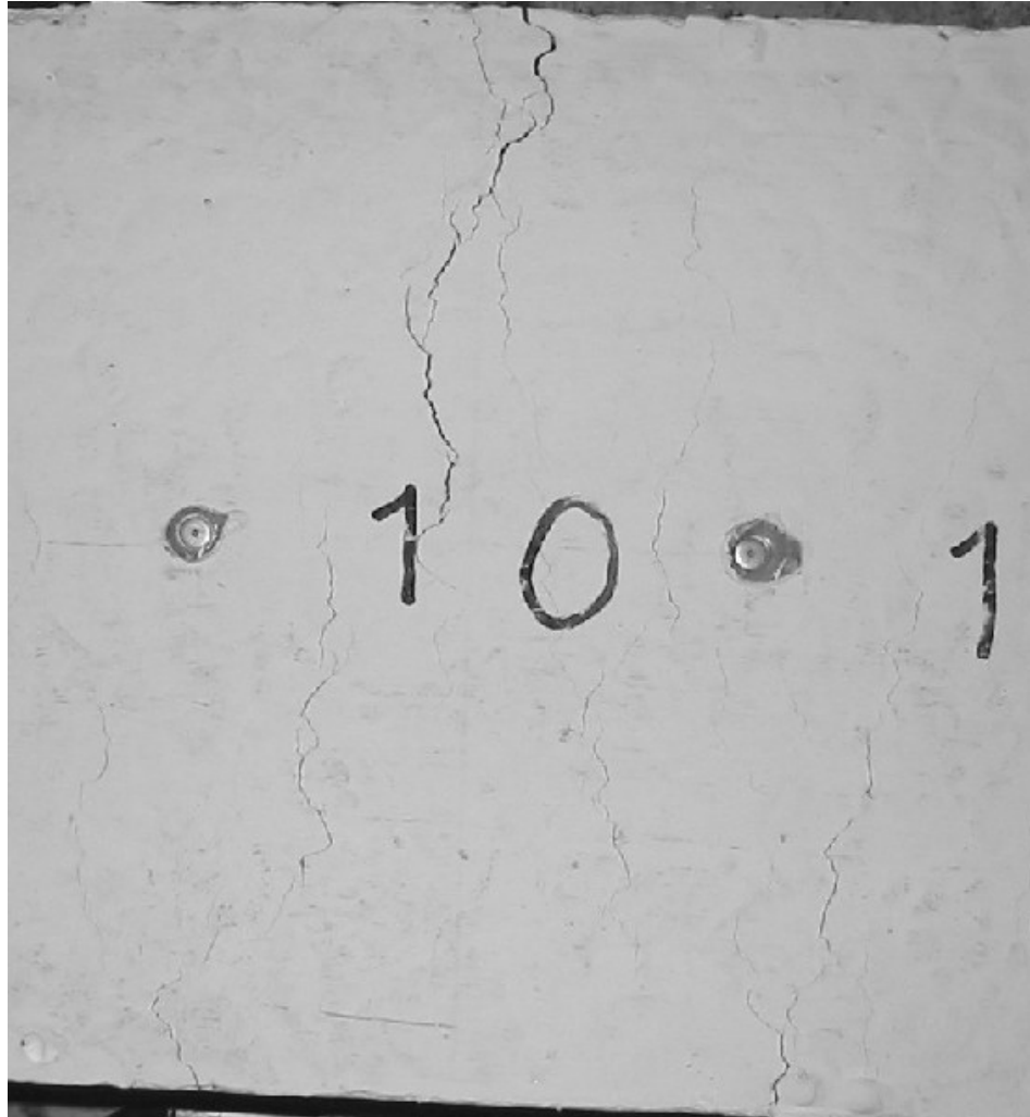
Figure 6.32 – Cracking pattern at the surface of the Glasgrid ® reinforced specimen at the end of the test (after 4 mm)
