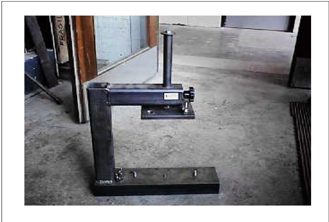
Figure 5.16: The jig used for fixing end plates
