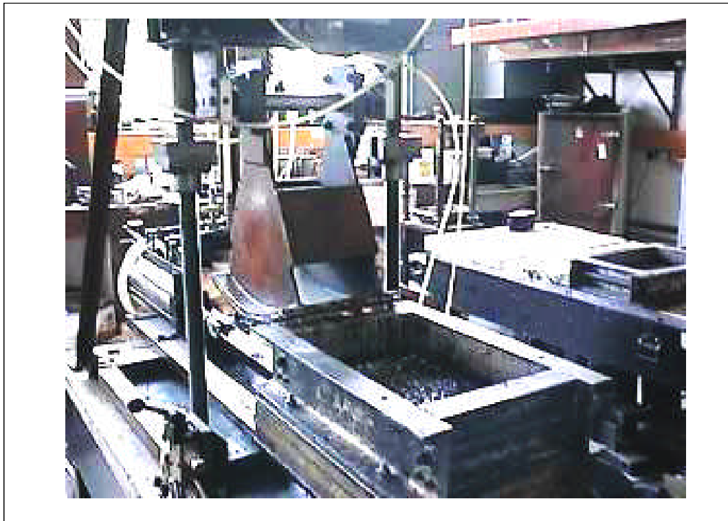
Figure 5.14: The rolling wheel compactor
