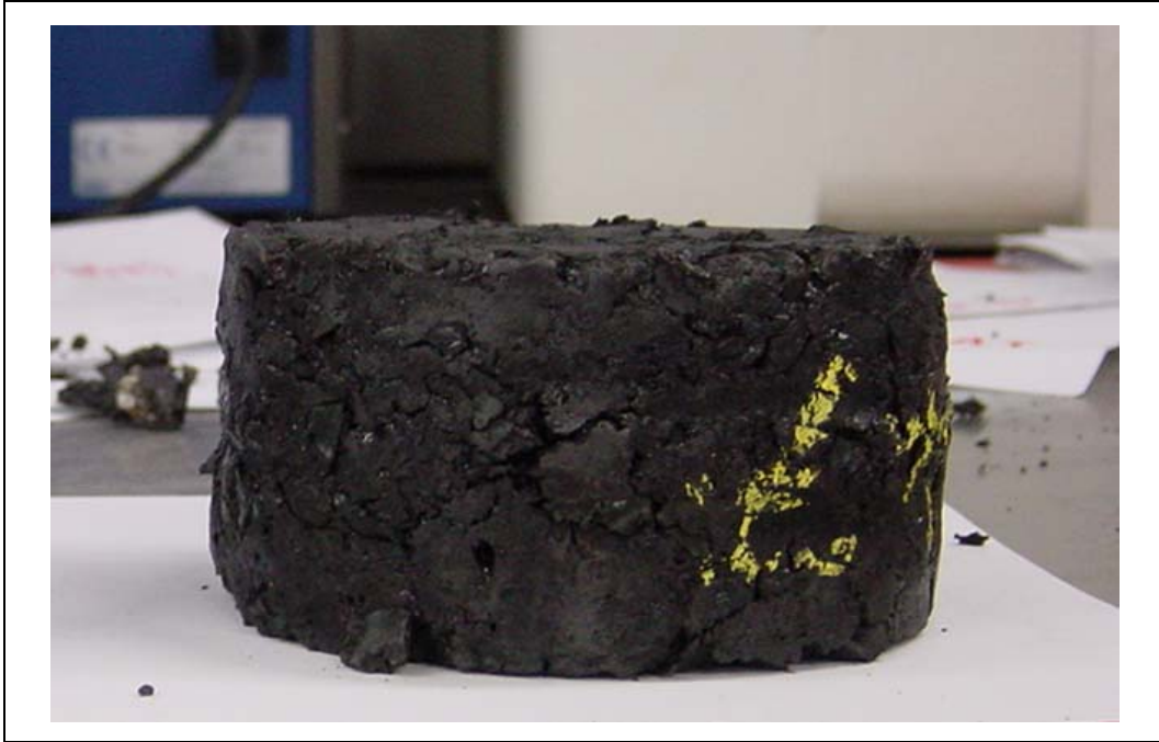
Figure 8.16: R5-C0-L specimen subjected to 2 hours pre-conditioning at 60 0 C prior to CRLAT testing and tested at 60 0 C with 70kPa confining pressure for 3600 seconds.
