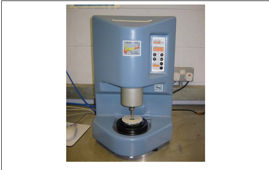
Figure 2.4: Bohlin Gemini dynamic shear rheometer
