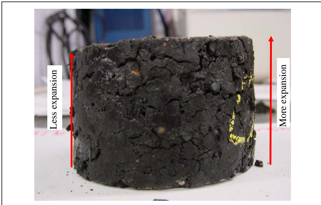
Figure 8.15: R5-C0-L specimen subjected to 2 hours pre-conditioning at 60 o C prior to CRLAT testing
