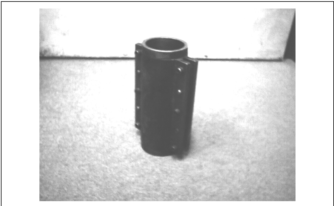
Figure 6.2: Split mould to produce rubber-bitumen composite specimens
