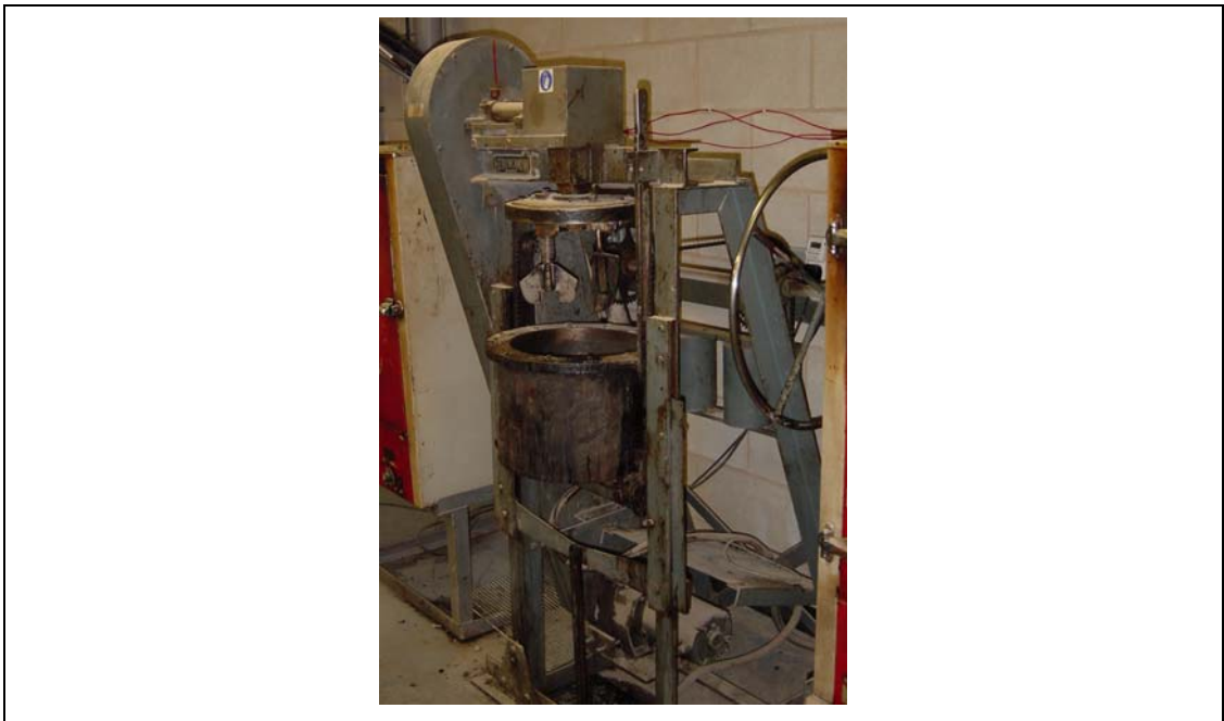
Figure 7.5: Sun-and-Planet asphalt mixer
