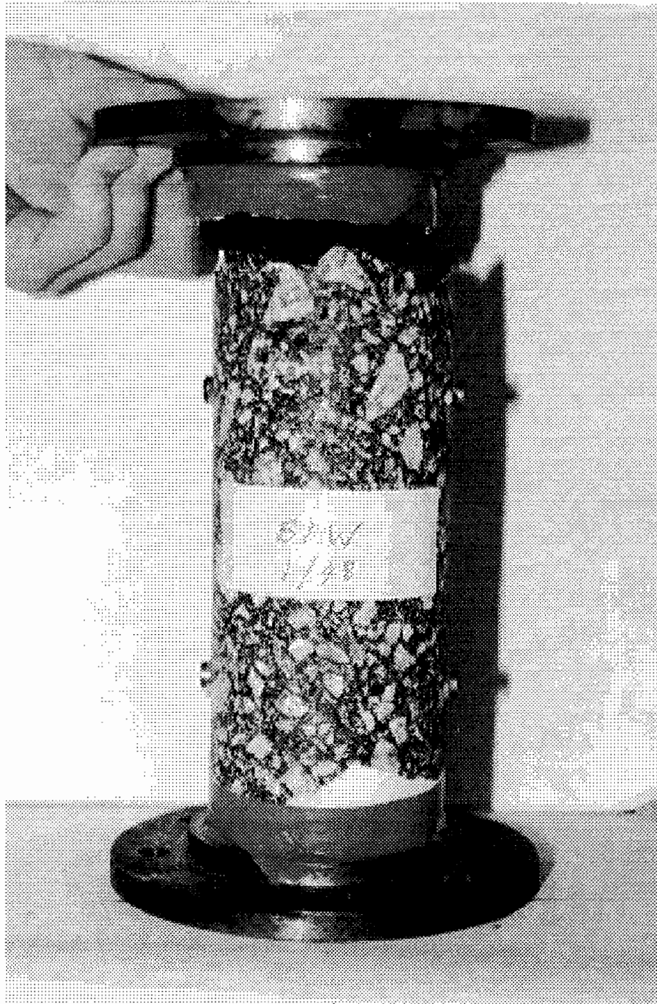
Figure 5.6 : Failed Specimen - Uniaxial Tension-Compression Fatigue Test
