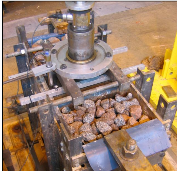
Figure 6.1 (b) The box test set-up
