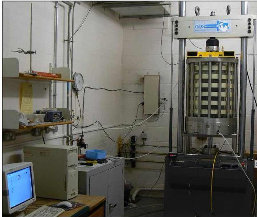
Figure 3.1 (a) Large scale triaxial apparatus testing system at the laboratory
