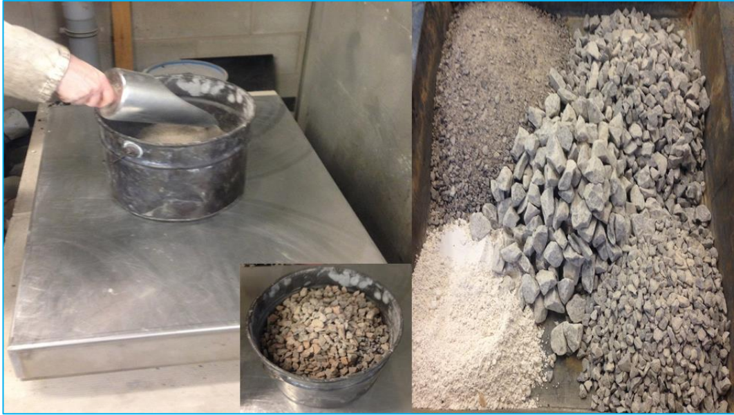
Figure 3.5: Batching process for aggregate
