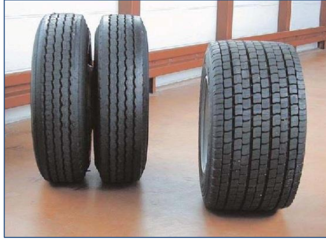
Figure 2.11: Dual-based vs wide-based tyre (Soares 2005)
