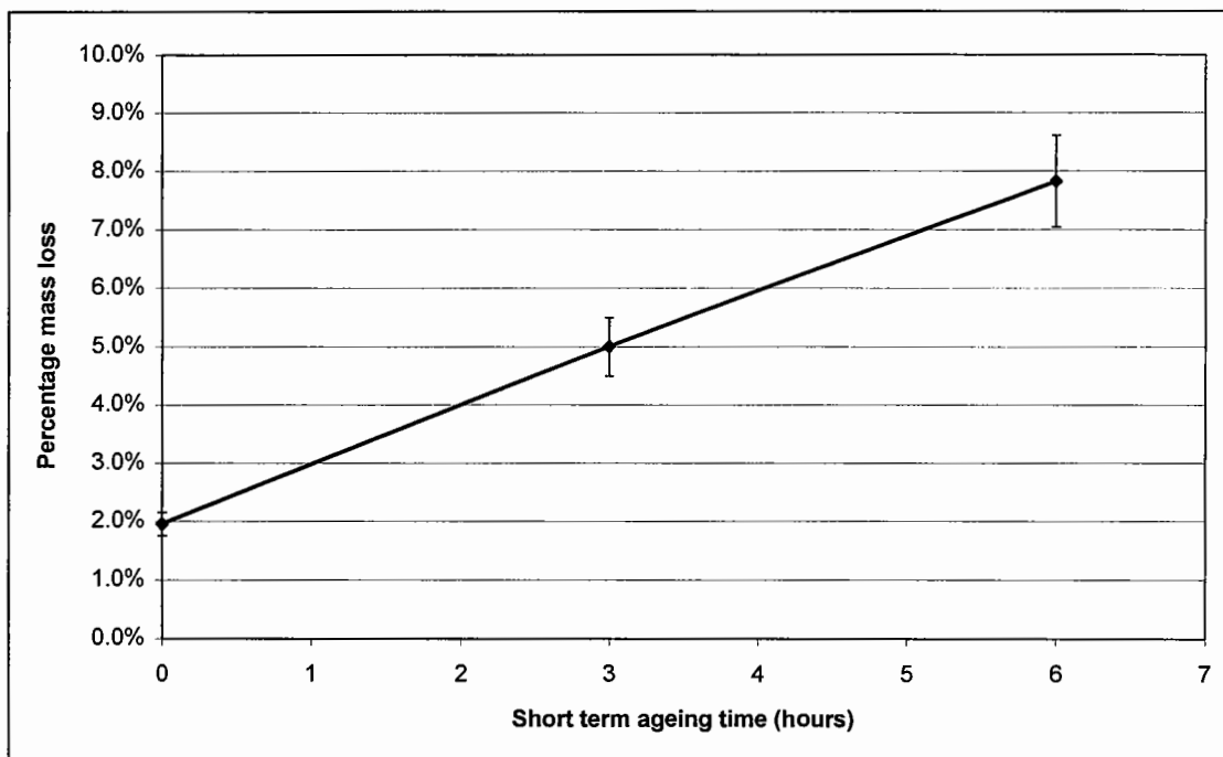
Figure 6.2 - Percentage mass loss of short term aged specimens of the original 3/20 IAA tested in the Abrasive Wear Test
