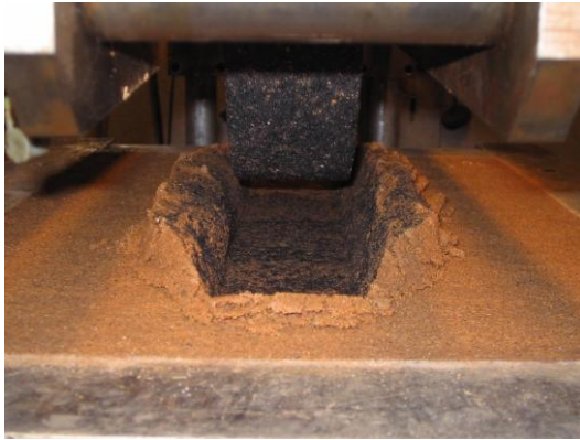
Figure 5. 5 Portaway Sand after 8000 passes with contact pressure of 100kPa using the SW
