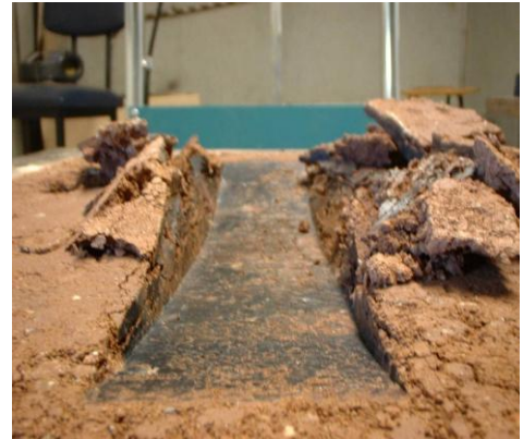
Figure 5. 6 Keuper Marl after 650 passes with contact pressure of 301kPa using the SW
