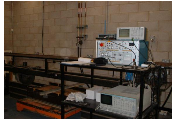
Figure 4. 6 The Nottingham Slab Testing Facility's control equipment
