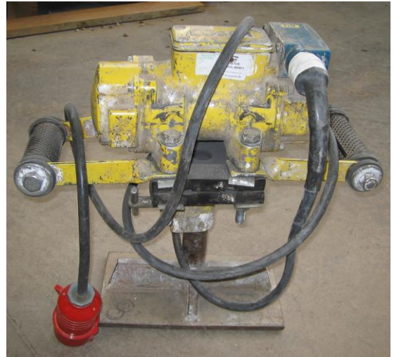
Figure 4. 10 Vibrating plate used on soils for the STF
