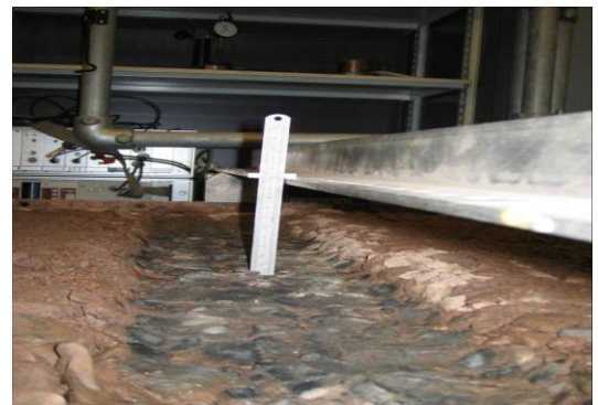
Figure 5. 8 Crushed Granite after 10000 passes with contact pressure of 355kPa using the STF
