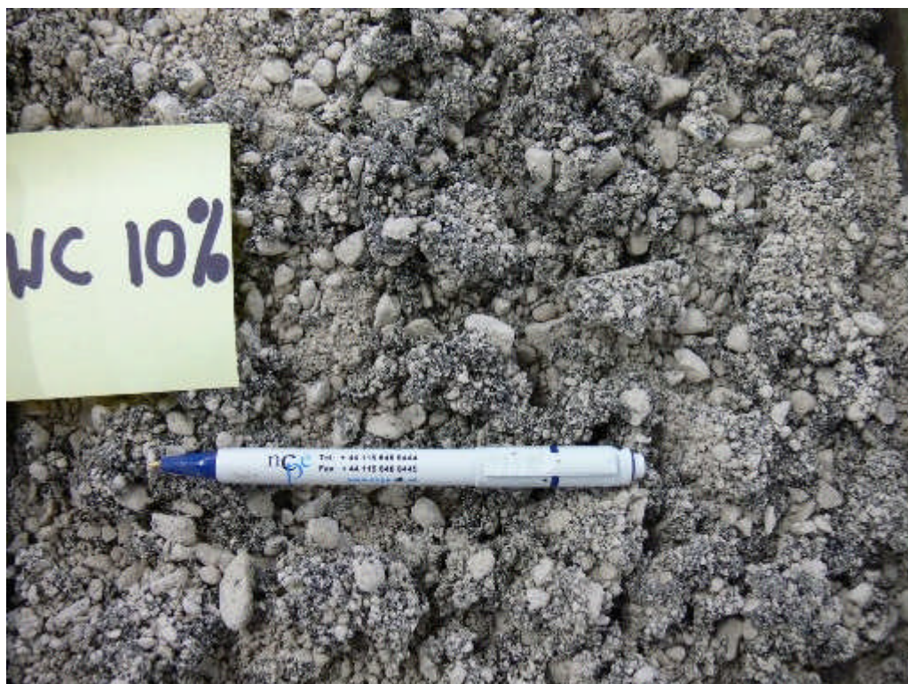
Figure A.6.9 – Appearance of binder distribution at 2 seconds mixing time of foamed asphalt mixture produced at a FWC of 10%.
