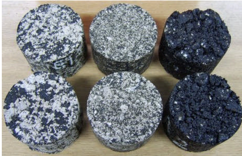
Figure 3.14 - Appearance of compacted specimens; (left) foamed asphalt mixed using spiral dough hook agitator, (middle) foamed asphalt mixed using flat agitator and (right) hot mix asphalt.
