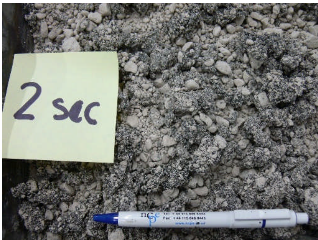
Figure A.6.3 – Appearance of binder distribution of foamed asphalt mixture at 2 seconds mixing time: forming large soft mastic globules
