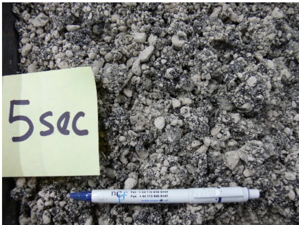
Figure A.6.4 – Appearance of binder distribution of foamed asphalt mixture at 5 seconds mixing time: forming broken soft mastic globules
