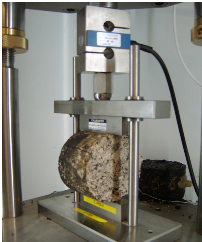
Figure 2.16 - Indirect tensile fatigue test (ITFT) configuration
