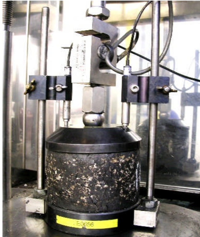
Figure 2.13 - RLAT test configuration using NAT apparatus
