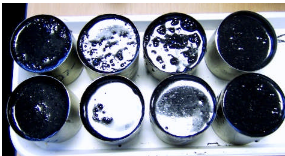
Figure 4.41 - Appearance of the collapsed foamed bitumen in the penetration test container.
