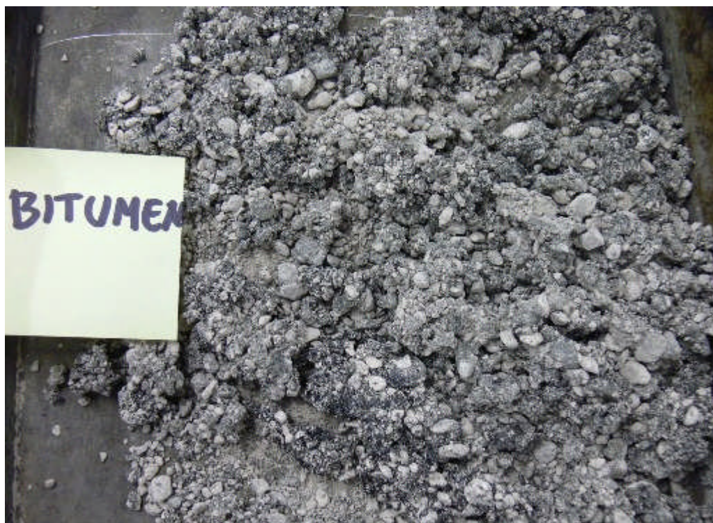
Figure A.6.1 – Appearance of binder distribution of hot bitumen sprayed into cold wet aggregates: the mixture is an uncombined asphalt, in which large stiff aggregate-bitumen globules occur.
