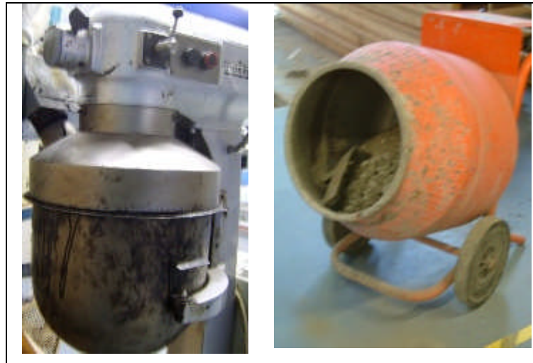
Figure 3.26 - Mixing process using Hobart mixer for foamed asphalt materials (left) and using concrete mixer for foamed asphalt plus cement (right).
