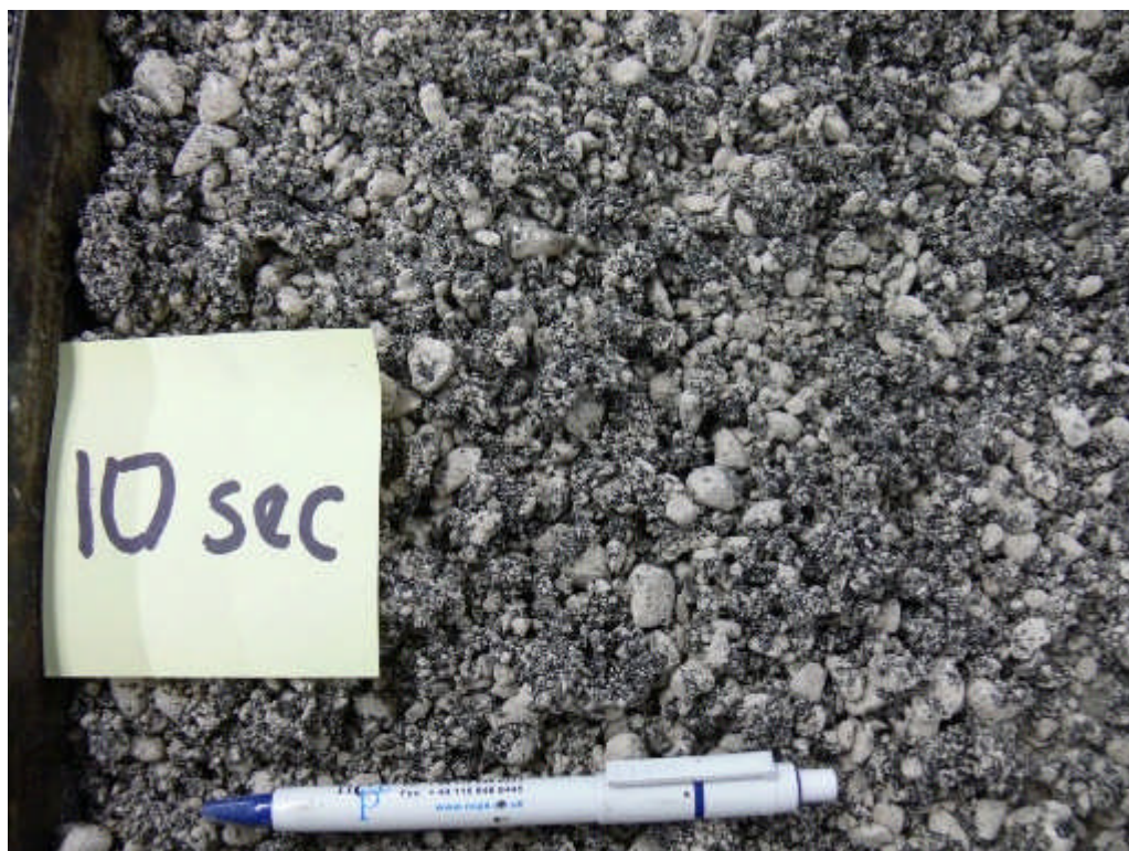
Figure A.6.5 – Appearance of binder distribution of foamed asphalt mixture at 10 seconds mixing time: forming binder-fines particles.
