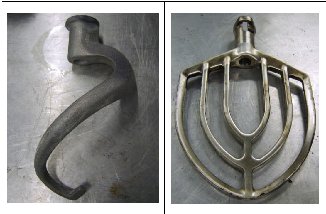
Figure 3.11 - Two types of agitator used in this study, Left: Spiral dough hook type; Right: Flat type
