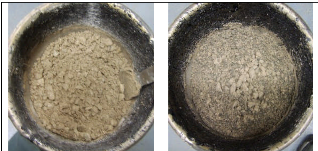
Figure 3.12 - Appearance of wet loose materials; (a) before foaming, (b) after foaming
