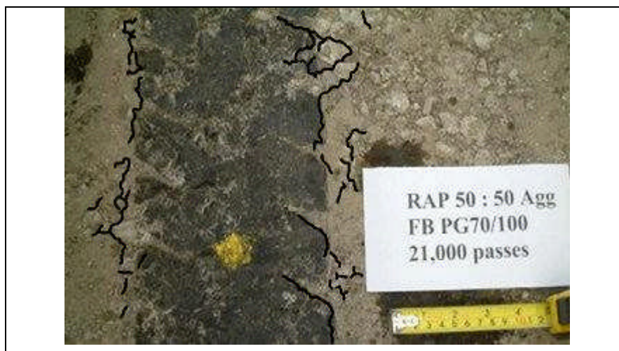
Figure 3.31 - Appearance of longitudinal cracks observed at both sides of the wheel path (coloured black).
