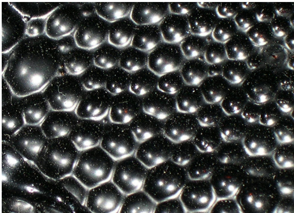
Figure 4.40 - Appearance of bubble structure of the collapsed foamed bitumen
