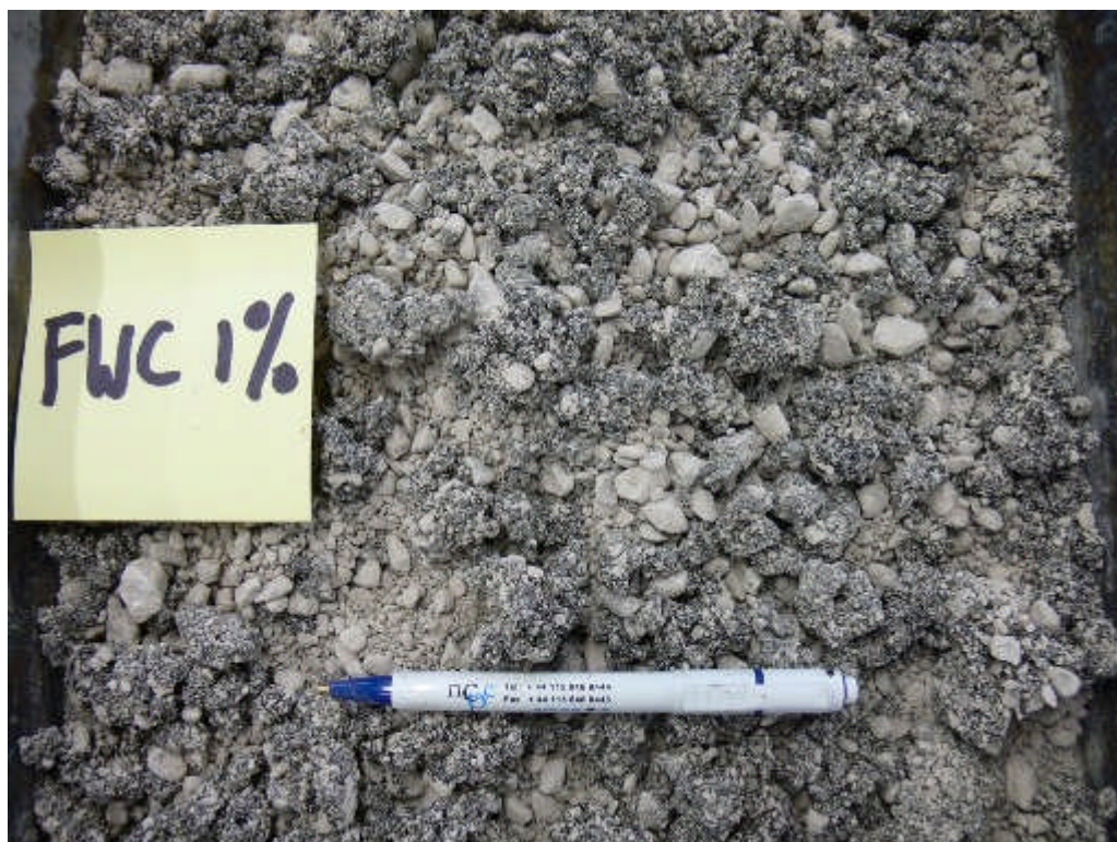
Figure A.6.7 – Appearance of binder distribution at 2 seconds mixing time of foamed asphalt mixture produced at a FWC of 1%.
