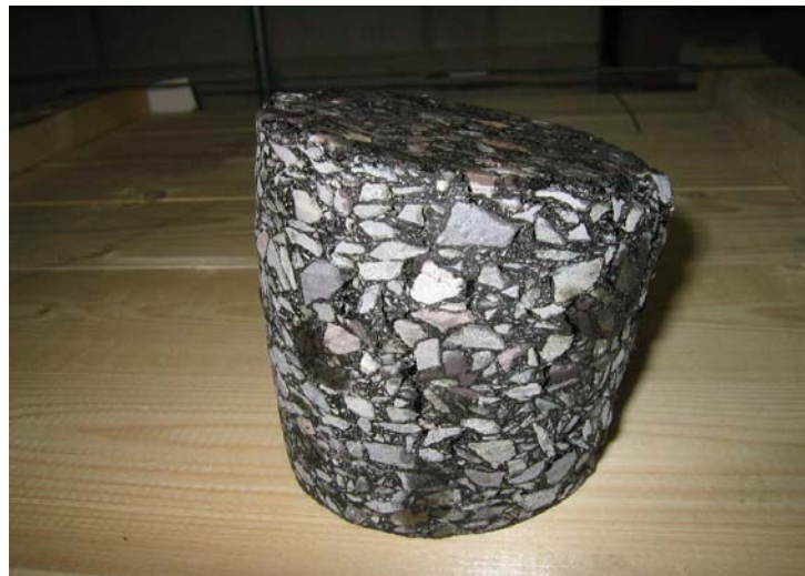
Figure 5.9 Specimen with more deformation on one side.
