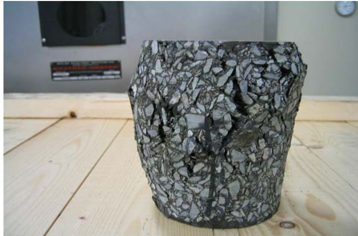
Figure 5.8 Specimen with more deformation in one end.
