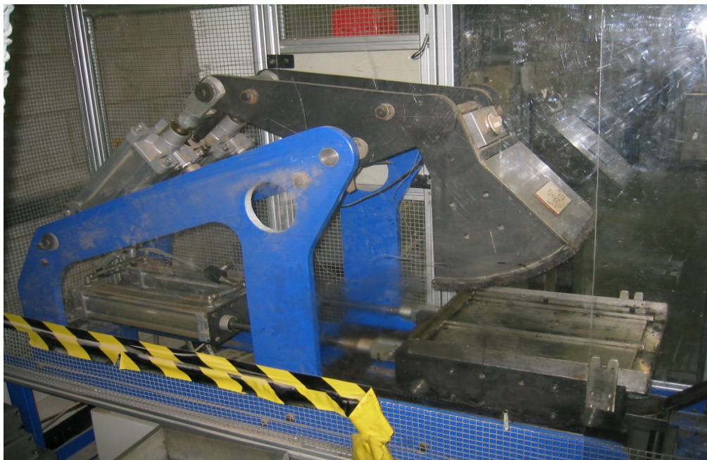
Figure 5.7 Laboratory roller compactor.
