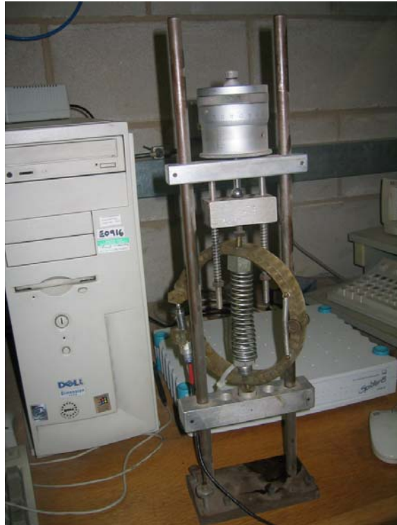
Figure 5.19 The set-up for calibration of radial LVDT.
