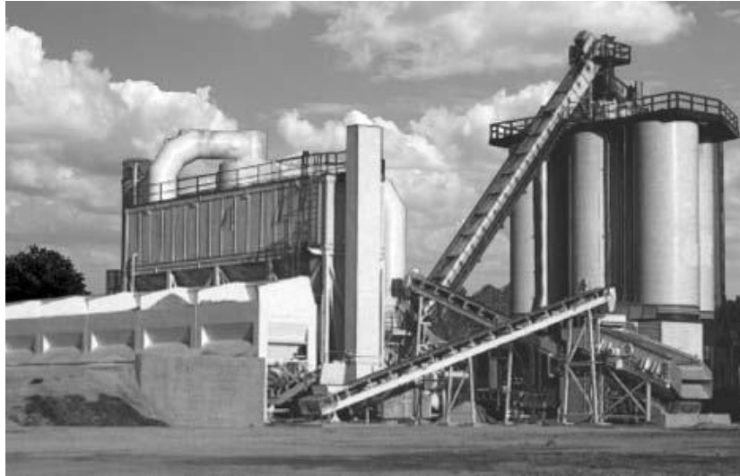
Figure 2-8 Asphalt batch plant with RAP infeed (ARRA, 2001)
