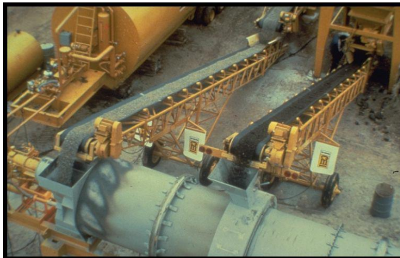
Figure 2-9 RAP introduction in asphalt drum plant (Kandhal and Mallick, 1997)
