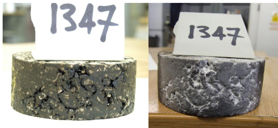
Figure 6-4 Distribution of voids on side surface of samples
