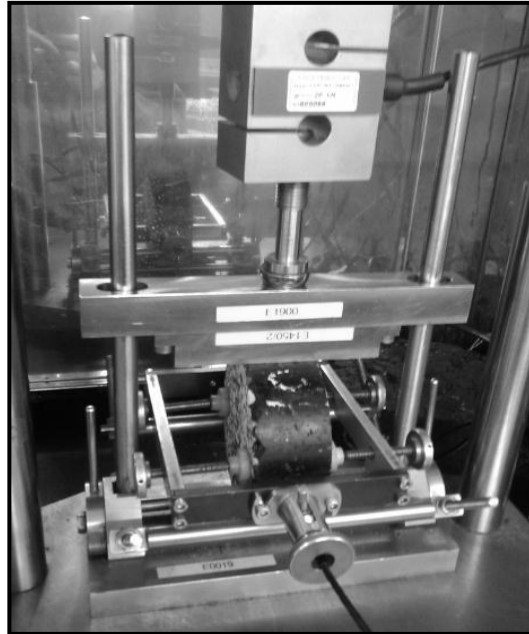
Figure 3-5 Indirect tensile stiffness modulus test
