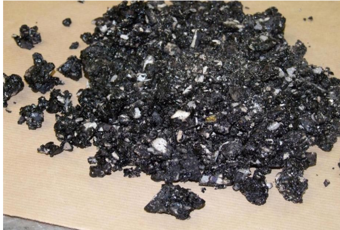
Figure 4-9 RAP particles after warming for 2 hours at 100 °C
