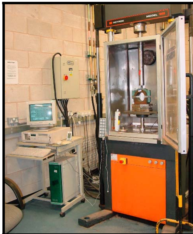
Figure 6.2: Instron machine arrangement for Marshall stability test
