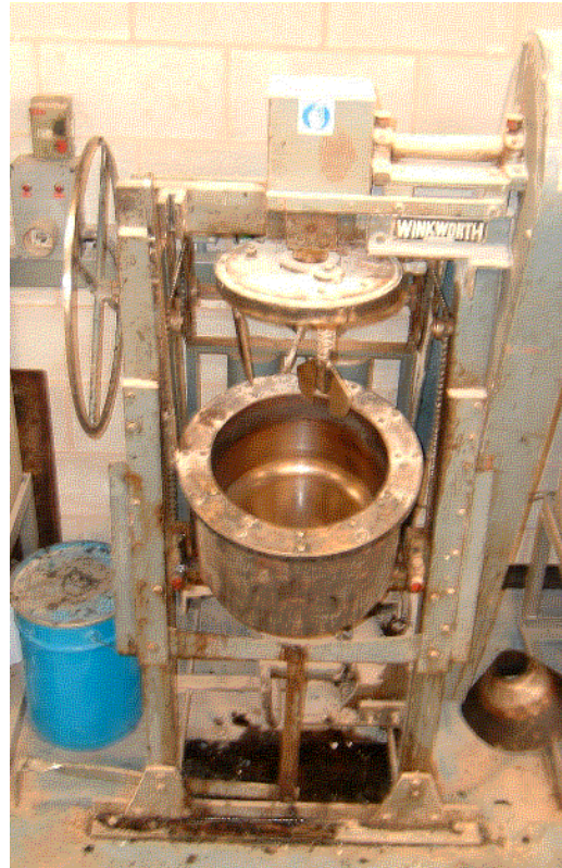
Figure 6.16: The mixer used for asphalt specimen production
