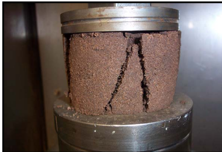
Figure 5.4: Performance test for determination of pozzolanic properties of tin slag
