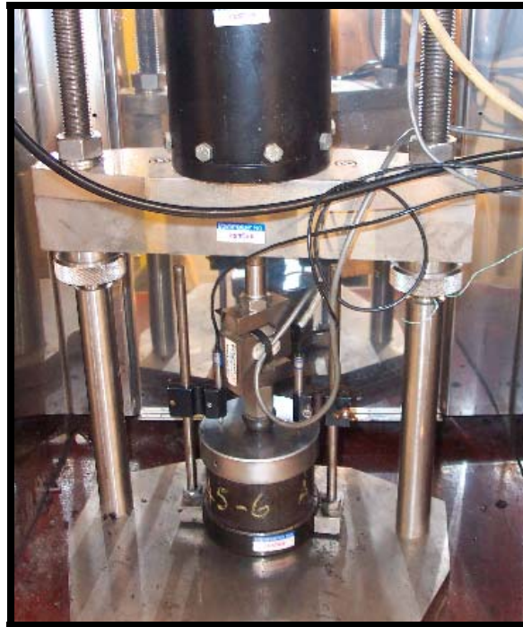
Figure 6.9: Repeated load axial test (RLAT) arrangement using NAT apparatus
