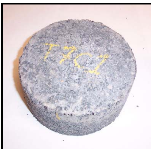
Figure 5.15: Cement Bound Material with tin slag and cement only
