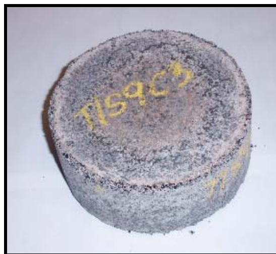
Figure 5.16: Cement Bound Material with tin slag/sand and cement
