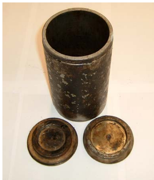
Figure 6.15: Gyratory Steel mould and end-plates
