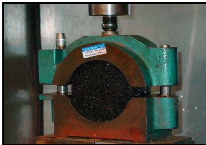
Figure 6.4: Marshall test head with specimen arrangement
