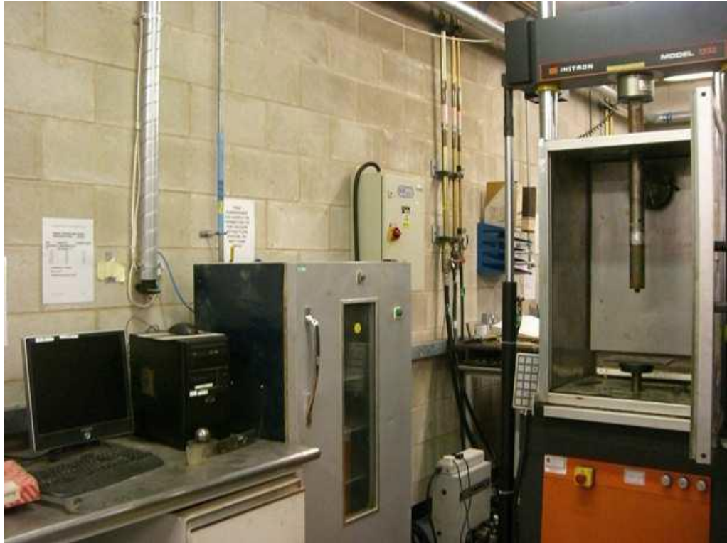
Figure 5.2 Uniaxial tests equipment – INSTRON (Taherkhani, 2006)
