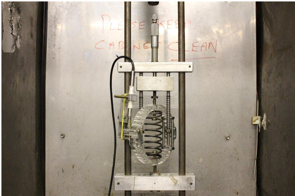
Figure 5.4 Caliper used to calibrate the LVDTs (axial strain)
