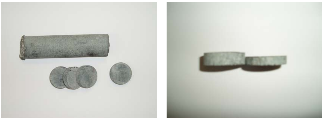
Figure B.4 Cutting and polishing of aggregate plates
