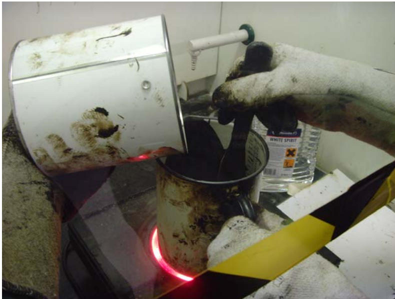
Figure 6.3 Picture of hand mixing of mastic
