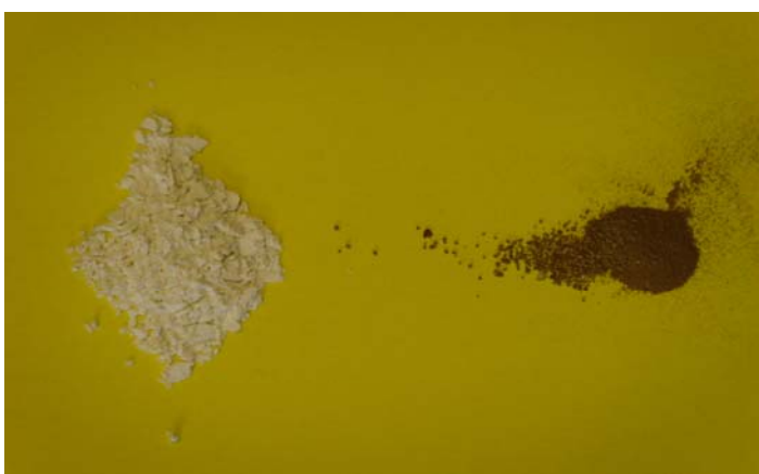
Figure 6.18 Comparison of original limestone filler (left) and the residual one from binder recovery
