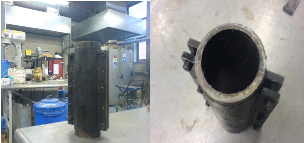
Figure 4.1: Photograph showing split mould.
