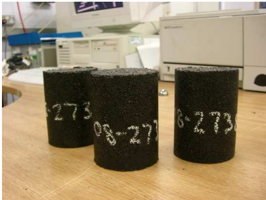
Figure 4.2: Photograph showing a typical specimen of idealised asphalt mixture.
