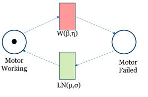
$q_{Motor}$ , failing to operate for 30 hours is 0.005839
