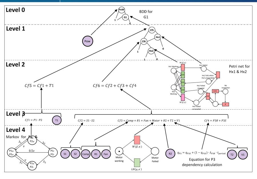
The function that represents system failure probability will be a function of probabilities taken from:
