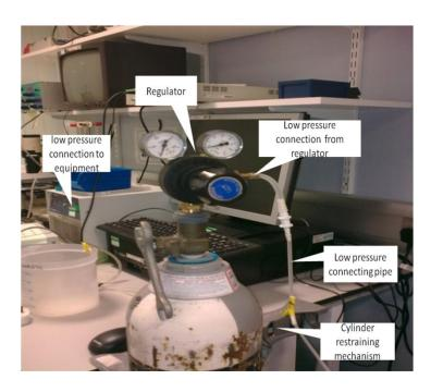
Guidelines for the inspection and maintenance of high & low pressure components associated with standalone compressed gas cylinders
