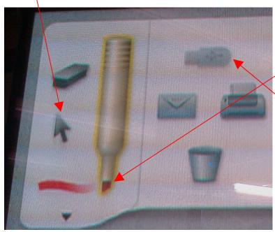
Use the real pen and tap this pen to get different colours. Drag pages onto the USB stick which you plug into the bottom of the system or tap the file menu and 'Save to USB stick'
